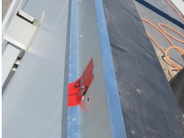
Figure 3.17: Cleat pressure tap (Courtesy of NRCC)
