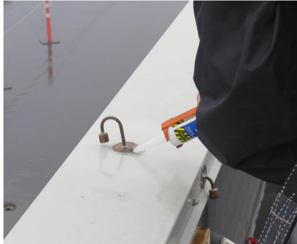
Figure 3.19: Applying epoxy to the pressure tap on the top face (Courtesy of Laith Hajsaid, University of Ottawa)
