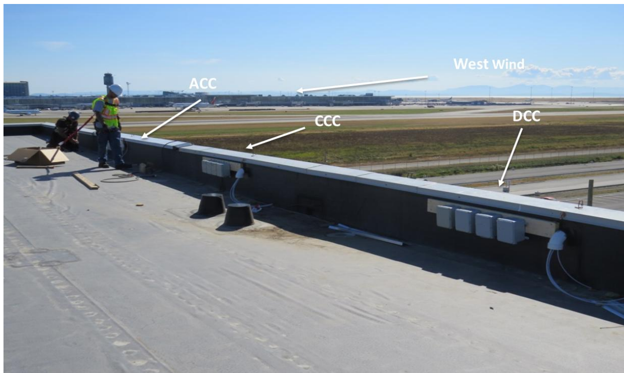
Figure 3.8: Instrumented edge configurations (Courtesy of NRCC)
