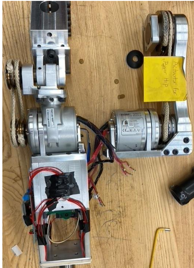
Figure 3.10 Front and lateral mount powered hip joints with customized top plates to directly attach to the chassis, bypassing the need for pyramid adapters.
