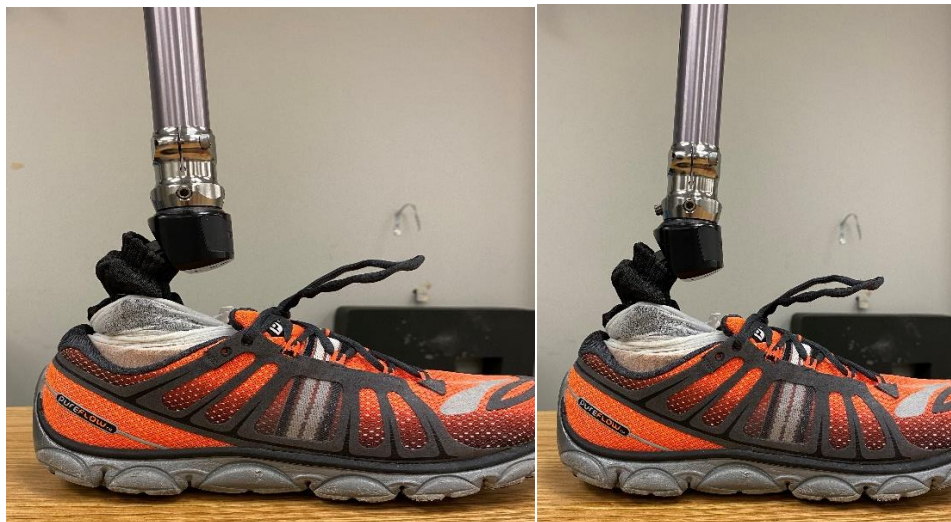
Figure 3.7 Pyramid adapter angle adjustments between the male pyramid adapter of an Össur Proflex XC foot and a pylon with a female pyramid adapter. From the pyramid adapter's neutral upright position (left), the pyramid adapter can provide \pm 10 degrees of angle adjustment in the sagittal (right) and front planes.
