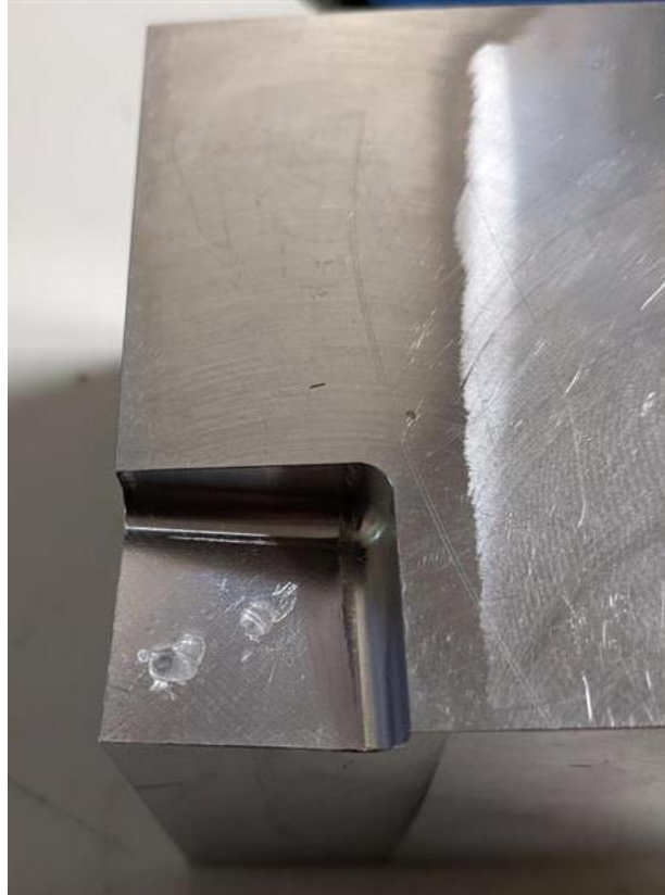
Figure 4.7 Observed deformation of the loading surface of the P5 LCI test rig after completing Instron load testing.
