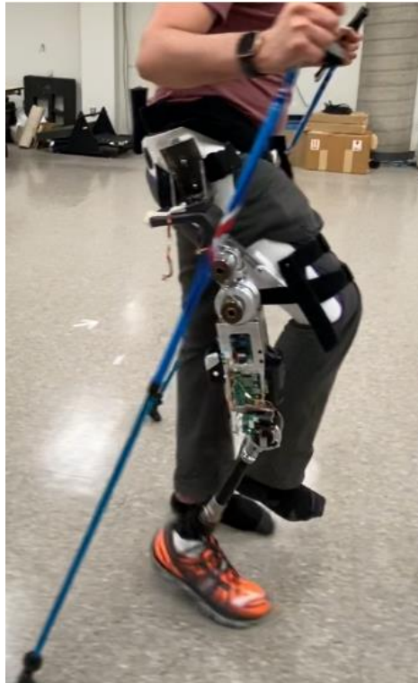
Figure 5.4 Toe drag observed during swing phase.
