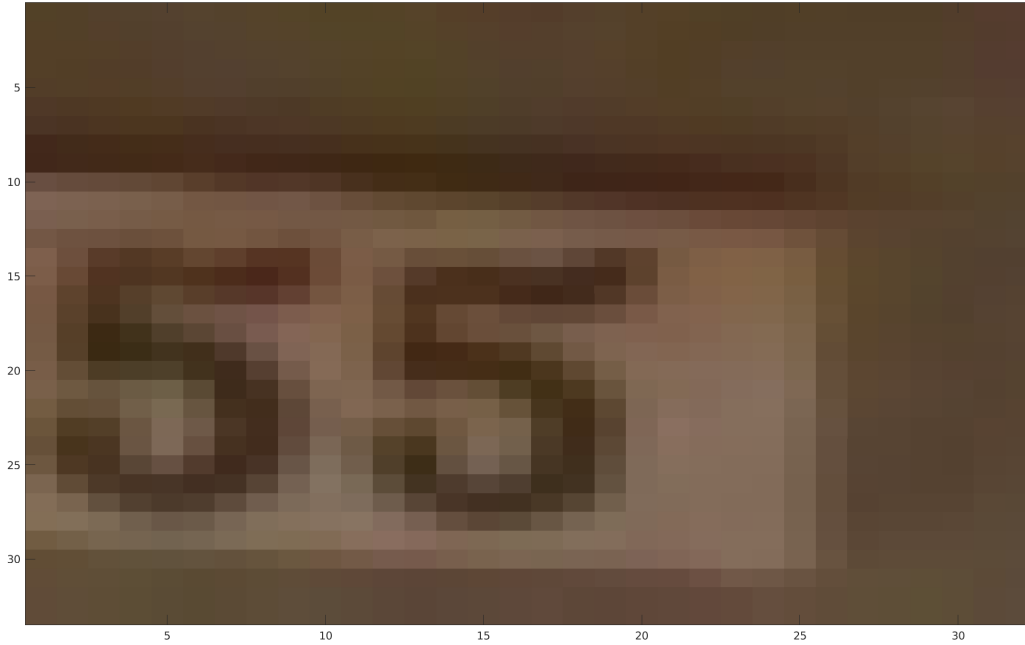
Figure 4.3: Example of an input X to a rank filter. The input is a 33 \times 33 RGB image \mathbf{X}_{33 \times 33 \times 3} .
