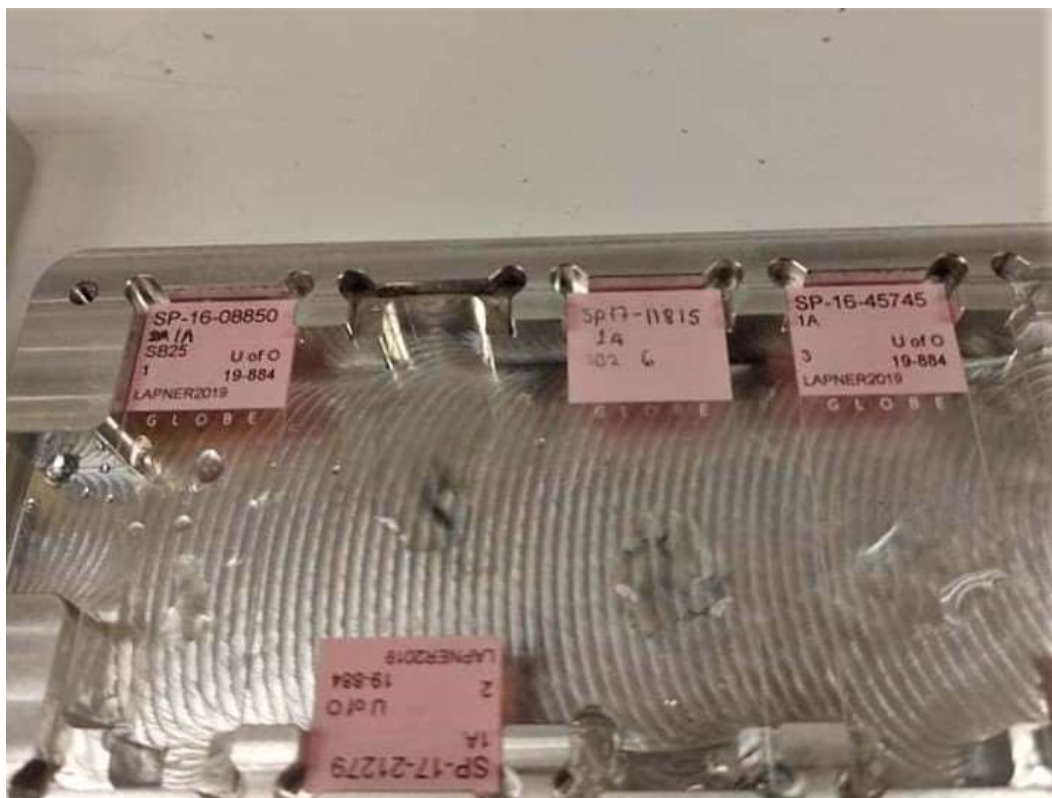
Figure 4.2: Slides in UV reactor slots after gold nanoparticle integration to the tissue samples.
