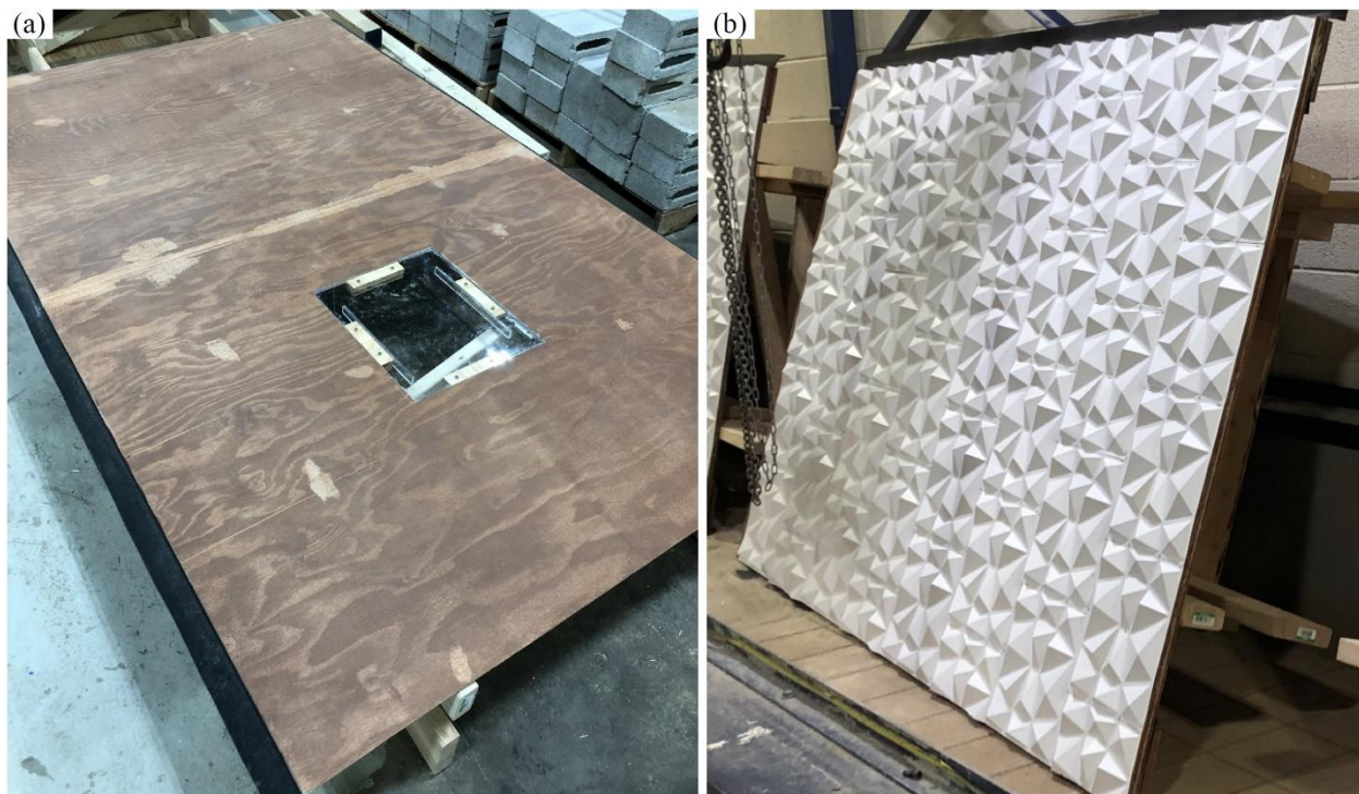
Fig. 6-3. Bottom surface of the ice cover: (a) smooth condition, and (b) rough condition.
