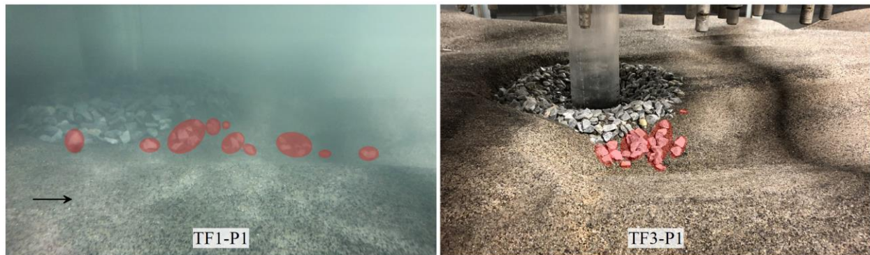
Fig. 5-10. Stone displacement photographs from TF1 and TF3 collected at the times specified in Fig. 5-8.
