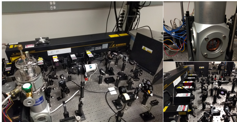
Figure 4.1: Photoluminescence measurement setup.
