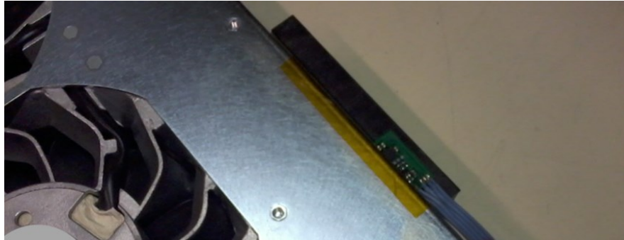
Figure 4.8: Accelerometer placement on long service life, unworn fan unit
