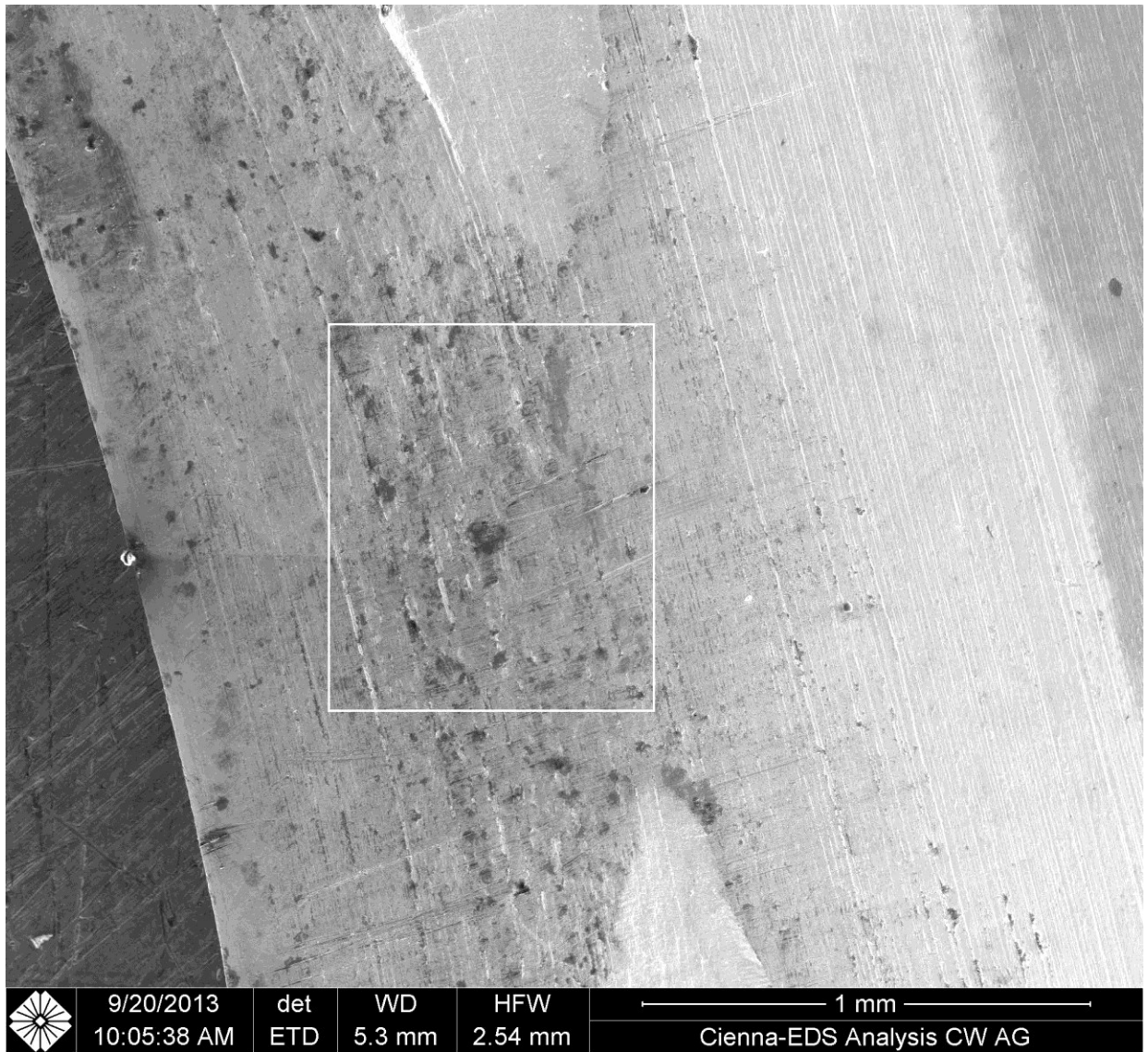
Figure 11.17: Male Power Blade #2 Regions Tested for EDX
