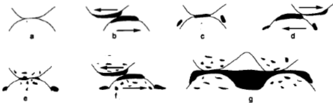
Figure 2.4: Stages of Fretting Corrosion [5]
