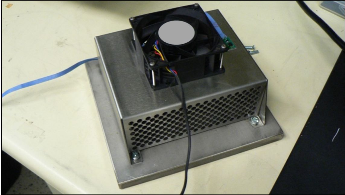
Figure 5.29: Individual Fan Test "Company_A" vs. "Company_B" Set Up Screwed Down Fan
