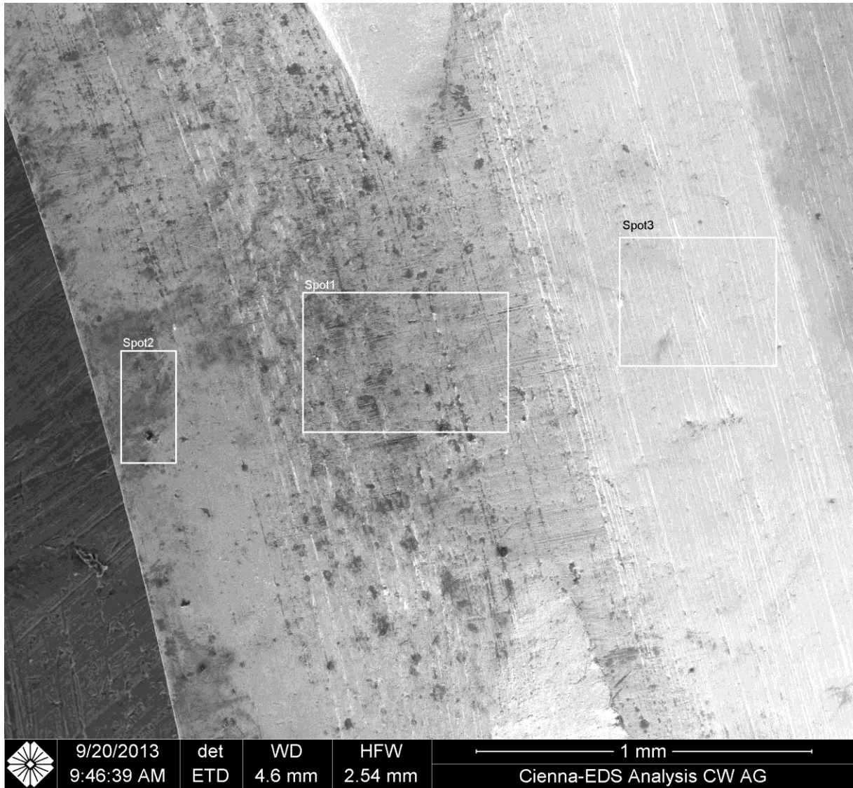
Figure 11.13: Male Power Blade #1 Regions Tested for EDX
