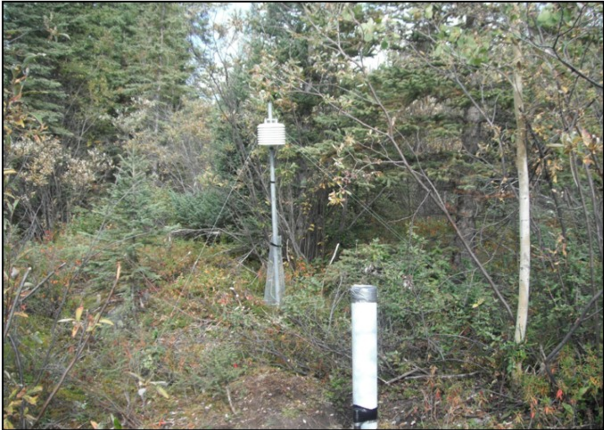
Figure 4.5: Climate station installed at Borehole R7 during summer 2011. Note the white radiation shield for the air temperature thermistor.
