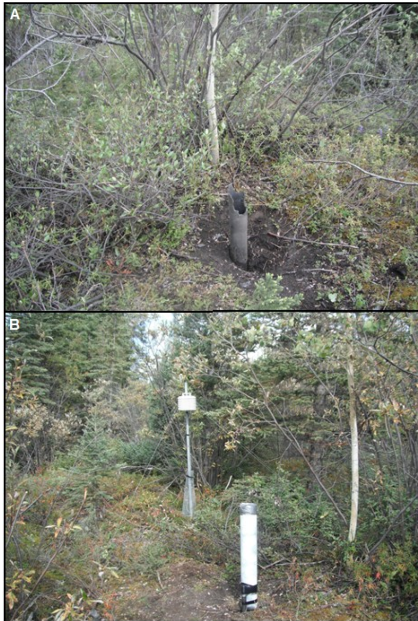
Figure 5.55: (A) Borehole R7 as it was found during the summer 2011 borehole exploration; (B) and borehole R7 after it was rehabilitated and cased.
