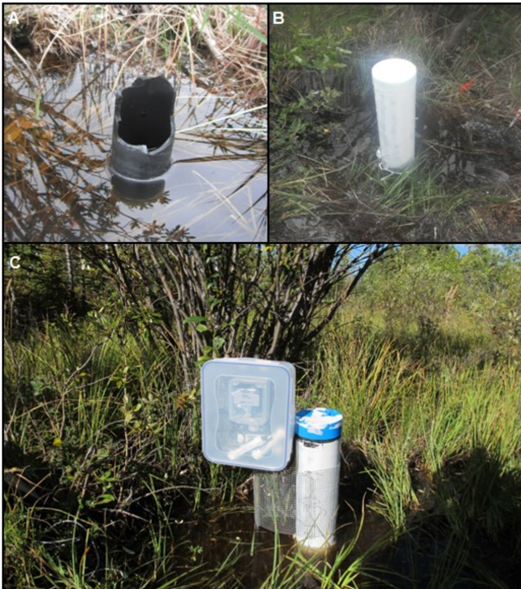
Figure 5.90: (A) Borehole H3 as it was found during the summer 2011 borehole exploration; (B) Borehole M4 after it was rehabilitated and cased in June 2011; (C) and Borehole H3 after it was instrumented with a HOBO H21-002 Micro Station in August 2012.
