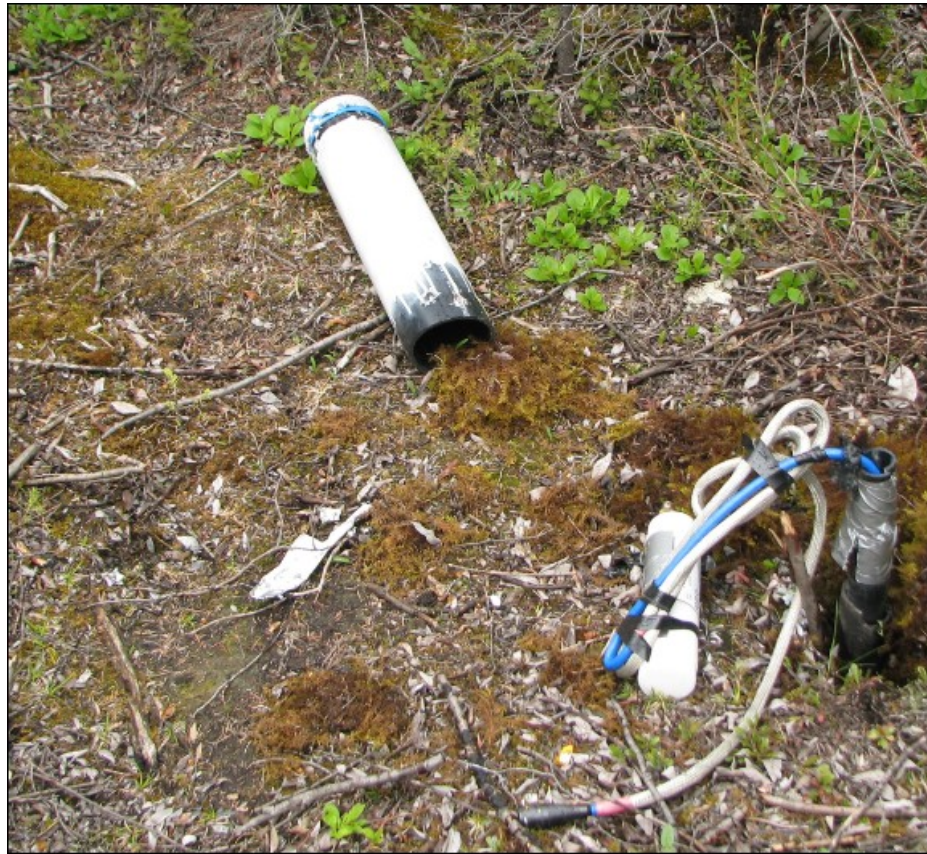
Figure 5.34: Borehole R4 on June 6, 2012. The borehole was found chewed by a bear and could not be repaired. The RBR logger record shows that the borehole was damaged on September 5, 2011.
