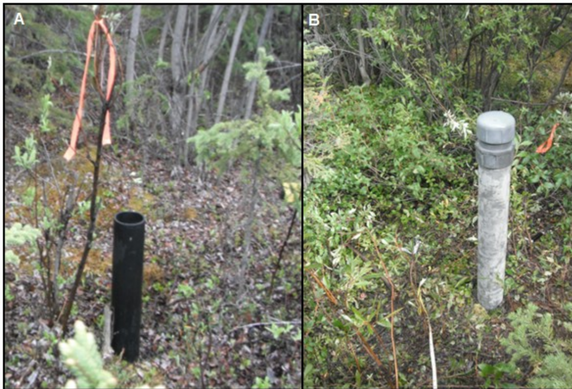
Figure 5.23: (A) Borehole R3 as it was found during the summer 2011 borehole exploration; (B) and borehole R3 after it was rehabilitated and cased.
