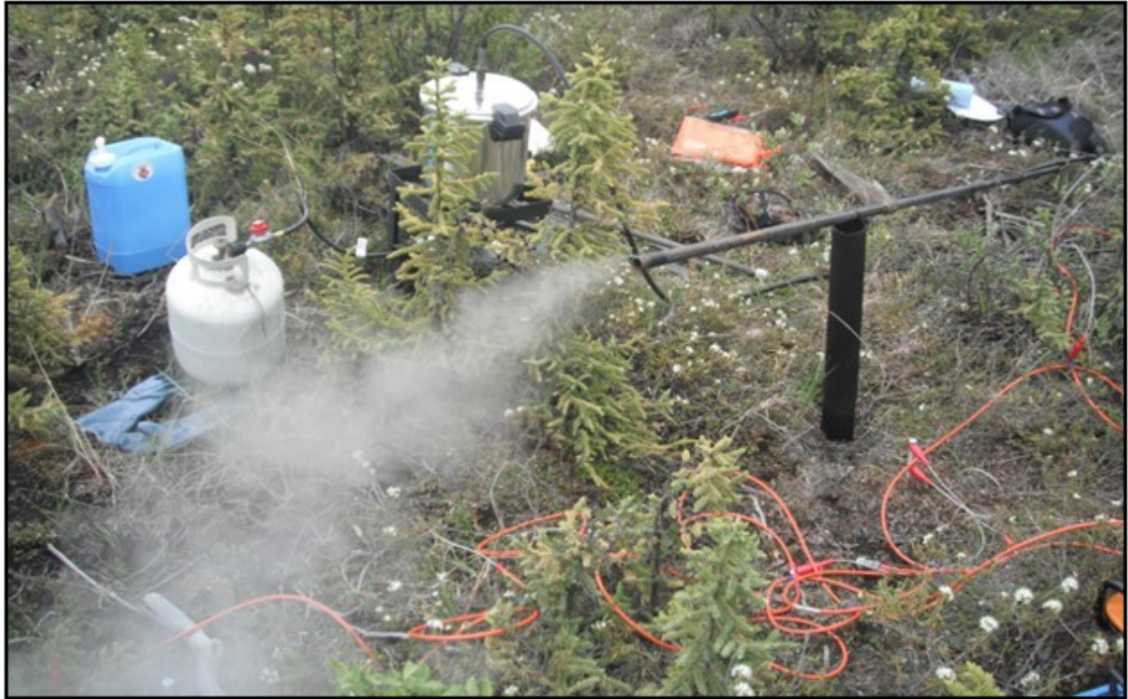
Figure 4.1: Custom-made portable steaming rig used to unblock boreholes of ice during 2011.
