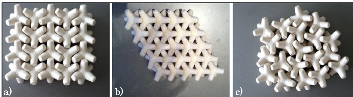
Figure 3: a) Uniform Rectangular Grid, b) Uniform Diamond Grid, c) Random Grid, all from Denechere (2009)
