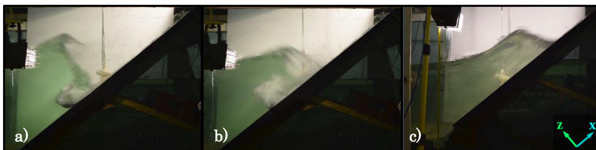
Figure 36: Example of Irregular Wave Breaking Characteristics - a) SSU_L1_Hs15_T1P2 b) SSU_L1_Hs15_TIP2, c) SSU_L3_Hs15_T1P8
