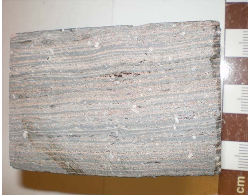
Figure 34: Drill-core sample ODC4, of core RDO-2A, from which slide #ODC-4 was cut. Note the mm-scale flow banding between light pinkish-brown and dark grey bands and the greater abundance of void space in the lighter pinkish-brown bands.
