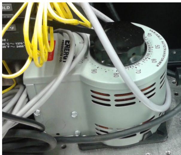
Figure 63: The variable autotransformer for the lightbulb inside the main chamber (left), and the thermocouple indicating the temperature inside the chamber (right). At the time when the picture was taken, the lightbulb was turned off.
