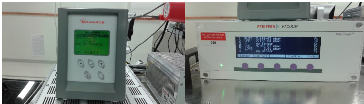
Figure 50: Pressure gauge of the mass spectrometer (Edwards, left) and main chamber (Pfeiffer, right)
