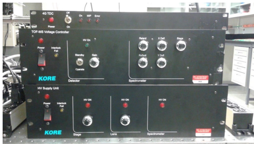
Figure 61: The three crucial units for the mass spectrometer and the pulsed extraction unit. The top unit is the Time to Digital Converter (TDC), the middle unit is the Voltage Controller and the bottom unit is the High Voltage Supply Unit.
