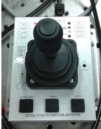
Figure 64: Joystick controlling one of the motorized mirrors in the main chamber. It can easily be connected to the other motorized mirror through the ports on the side of the chamber (Figure 65).
