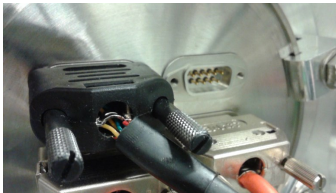
Figure 65: The ports connecting the joystick controller to the motorized mirrors inside the chamber. In the figure, it is connected to the first motorized mirror in the beam path.
