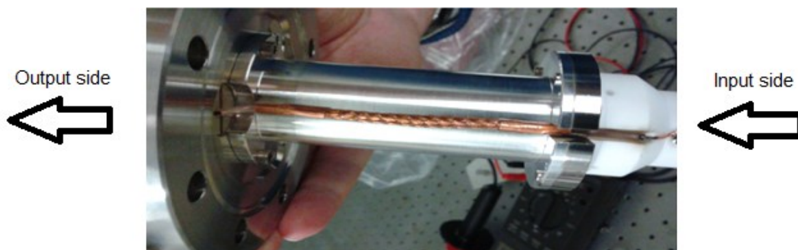
Figure 15: The lens system outside of vacuum, with the grounded funnel not attached. The funnel would normally be over the insulator (in white on the right). Repairs were done on the wire near the insulator. This is discussed more at figure 17. The wire connects the active element underneath the insulator to the voltage controller. The length of the tube after the insulator is grounded as well.
