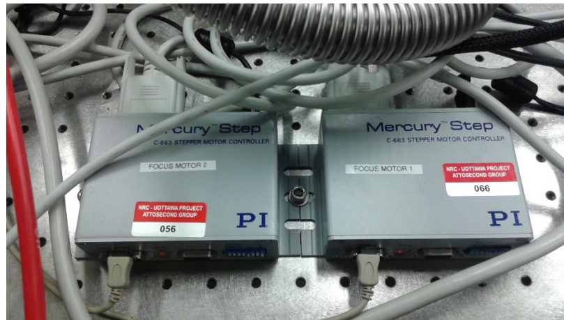
Figure 58: Both PI Stepper motors for the translation of the focussing objective beneath the sample and substrate inside the chamber.
