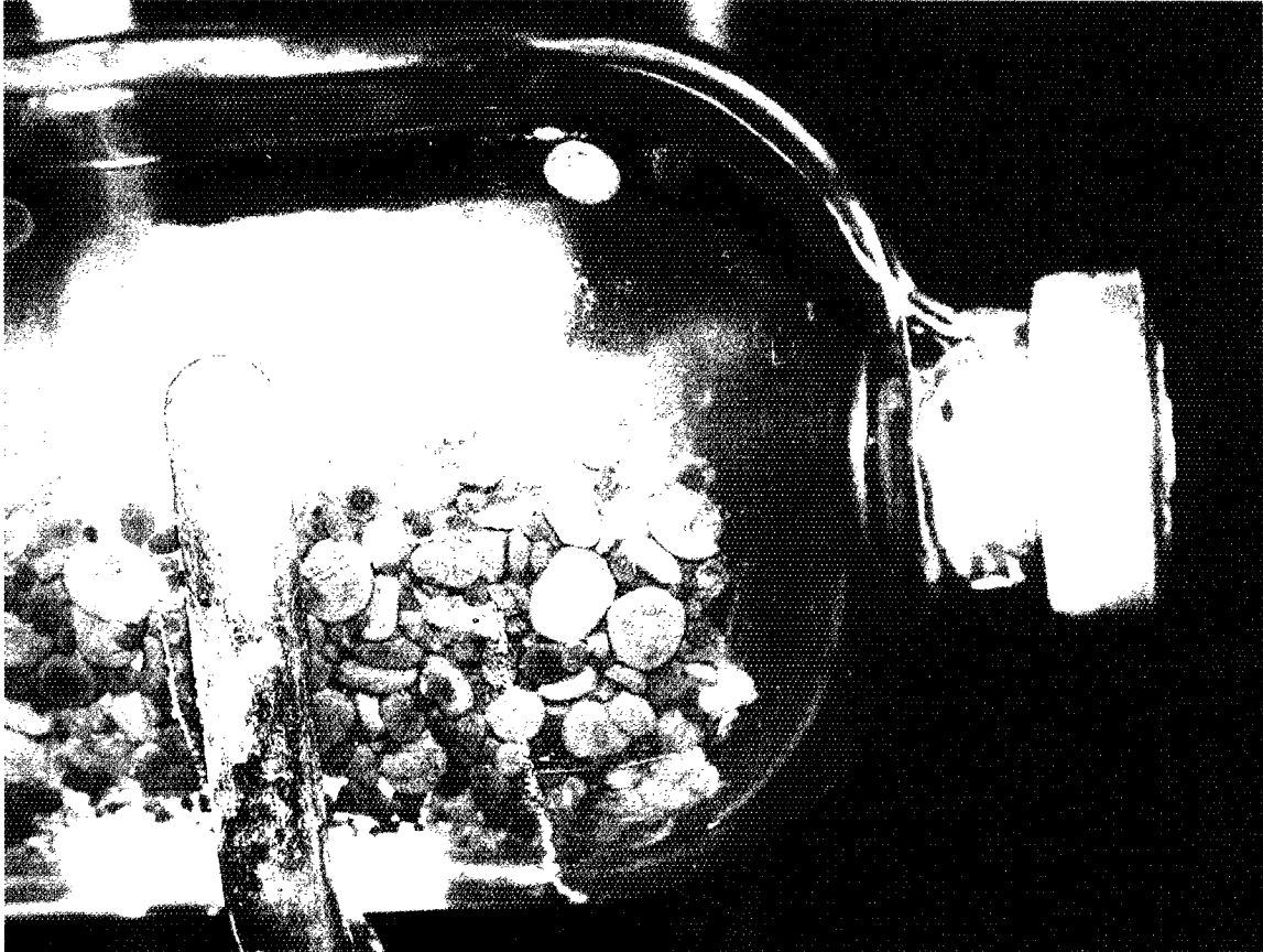
Figure 4.24: Biomass sample taken from compartment 2 of ABR operated without recycle at the end of the run period
