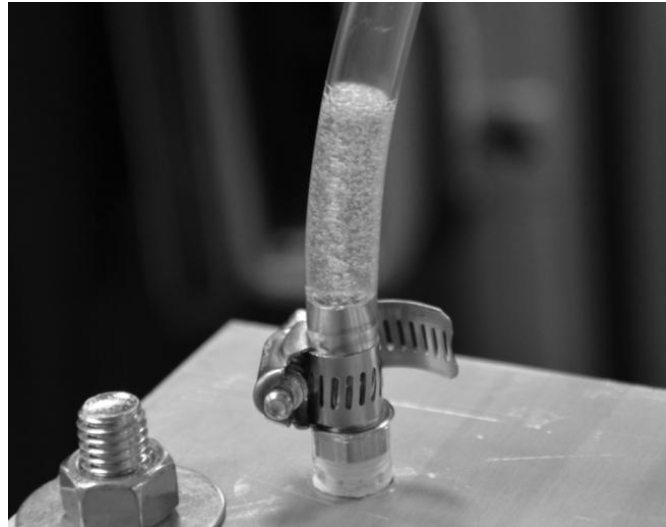
Figure 2.36: Air bubbles leaving the mould
