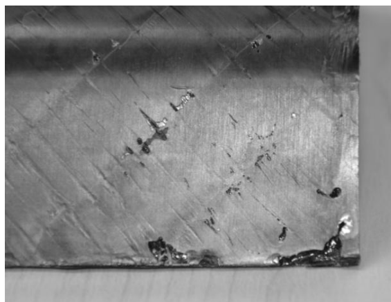
Figure 2.45: Dry spots in the vicinity of a vent
