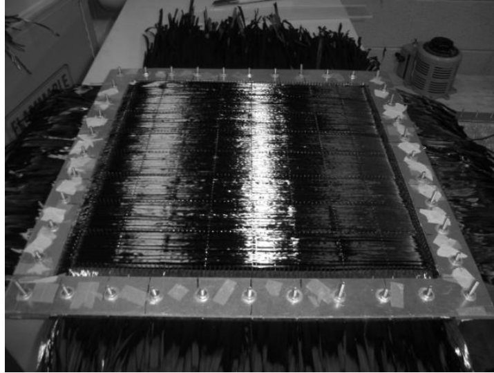
Figure 2.4: Clamped preform still in the pin-board
