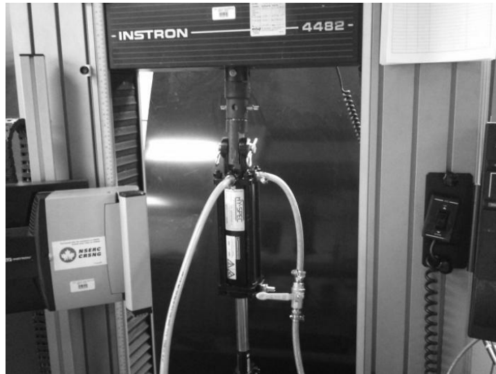
Figure 2.13: Hydraulic cylinder mounted on the INSTRON machine
