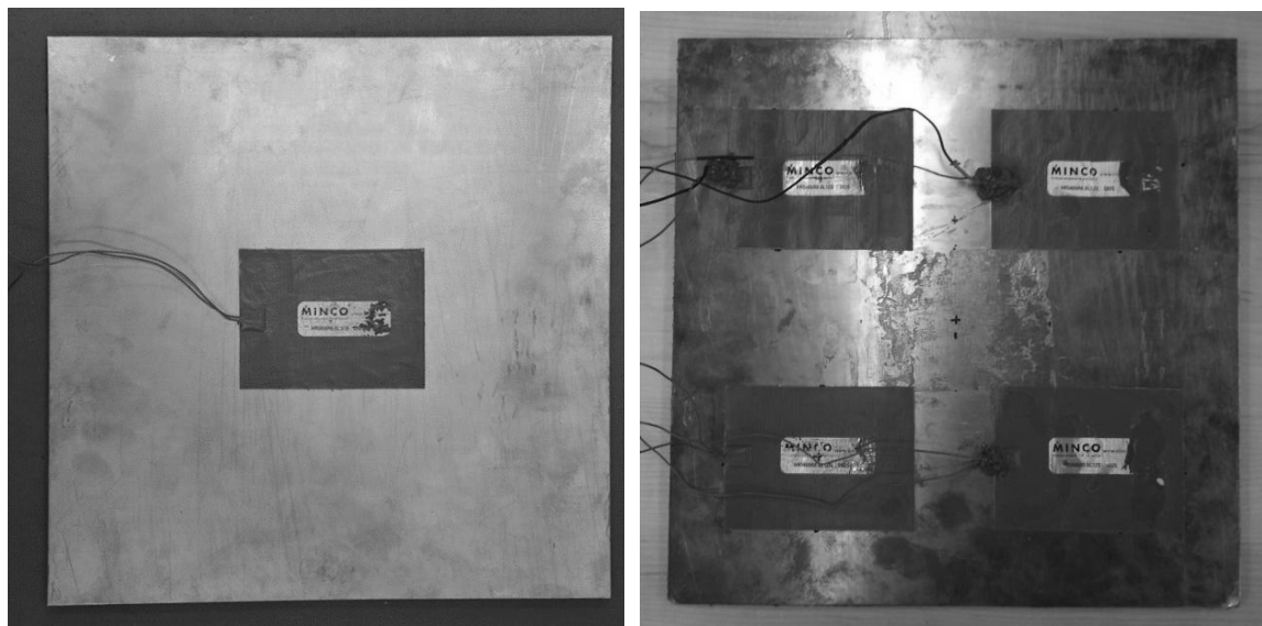
Figure 2.80: Heater configurations of the duplicate IHCT assembly
