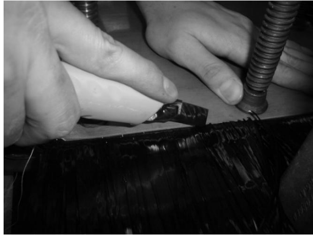
Figure 2.31: Cutting of dry preform using a snap-off blade
