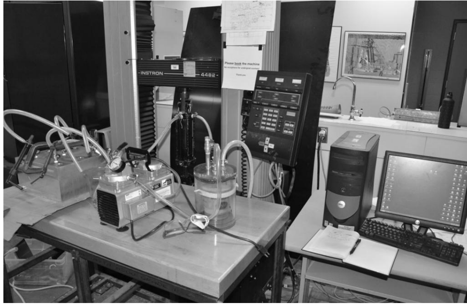
Figure 2.12: RTM injection setup
