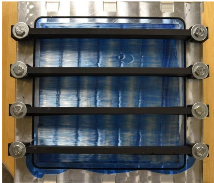
Figure 2.25: Top view of the infused preform
