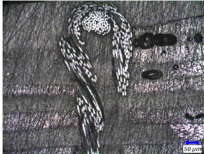
Figure 2.50: Micrograph of the vicinity of a stitch
