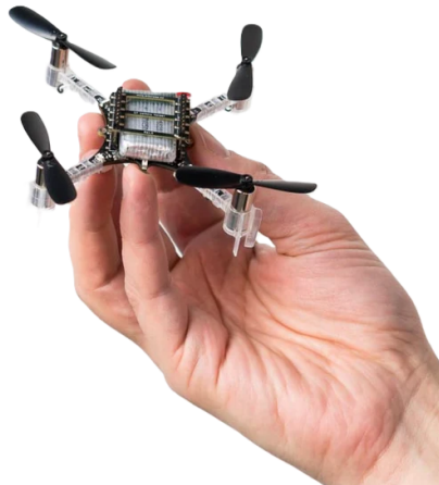
Figure 4.2: Crazyflie 2.1 Nano Quadcopter
