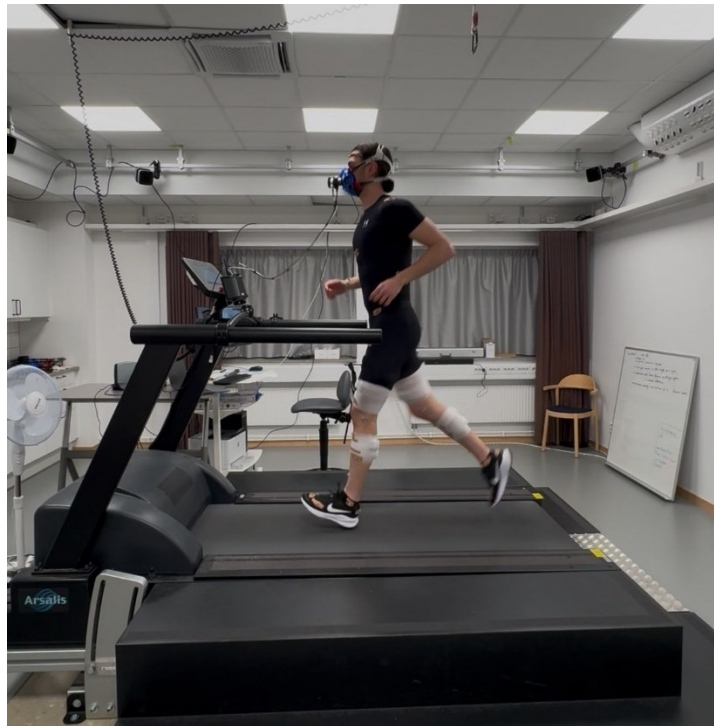
Figure 3.1: Experimental setup of HP COSMED with K5
