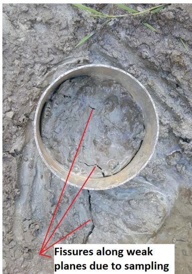
Figure 40. Distressed brittle Champlain sea clay during sampling
