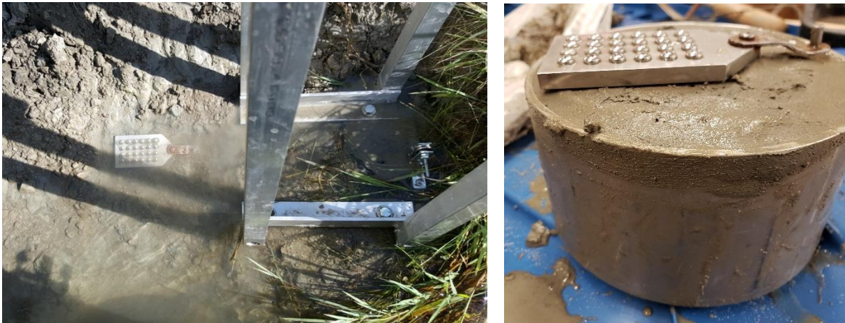
Figure 27. Erosionmeter probe deployed in the field and in the laboratory
