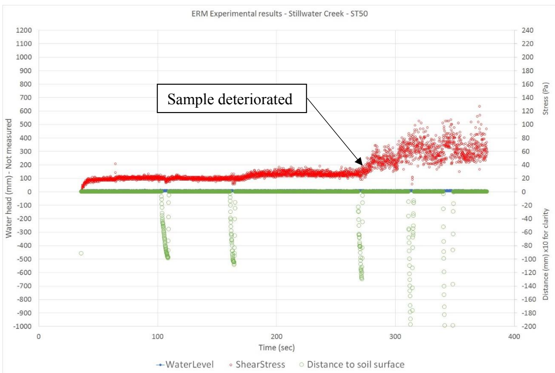
Figure 106. ST50, shear stress and distance measurements.
