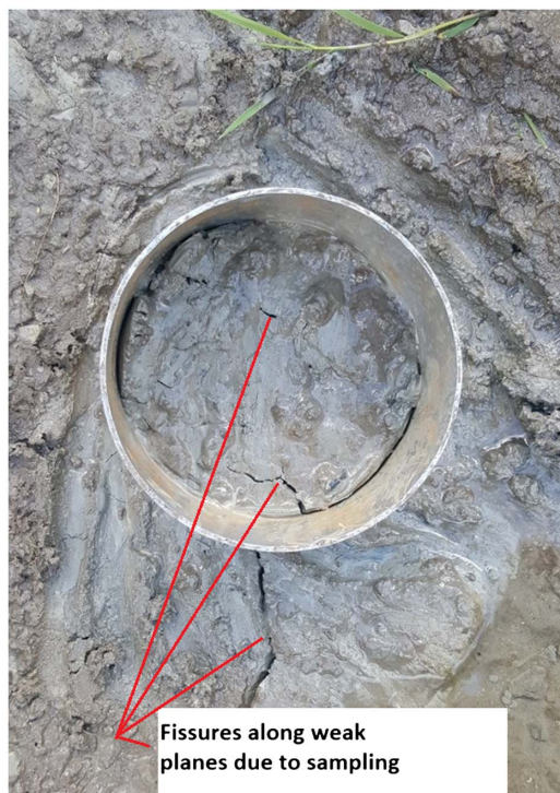
Fig. 10. Distressed brittle Champlain sea clay during sampling
