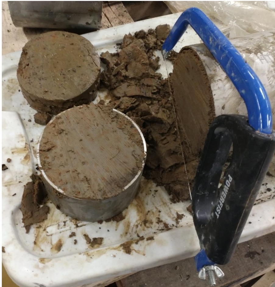
Figure 48. Specimen preparation – South Nation River #2
