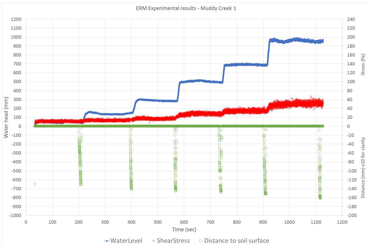
Figure 87. Muddy Creek sample, head, shear stress, and distance measurements.
