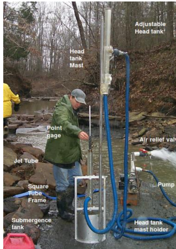
Figure 11: The original Jet apparatus deployed in the field, Hanson and Cook (2004)
