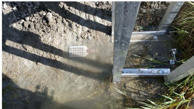
Fig. 2. Erosionometer deployed in the field
