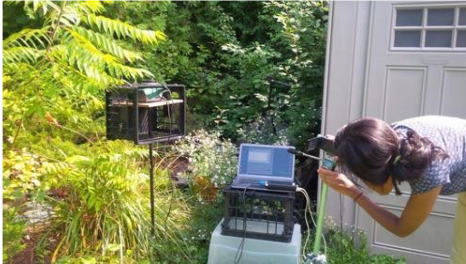
Figure C1. Experimental set up of outdoor feeder experiments. The sensor-activated feeding dish was placed on top of a platform containing the speaker located below. The speaker was connected to a laptop with pre-loaded defence sounds for playback when the sensor was triggered by a bird pecking at the disk. Before trials started a tarp was placed over the laptop. A video camera was placed ~1 m away from the platform to record the reactions of the birds.
