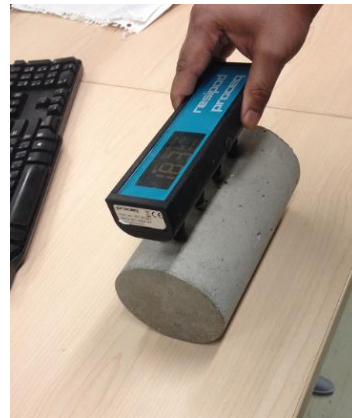
Figure 3.6. NDT test Setups performed on different RCA concrete mixtures presenting distinct qualities. A – UPV Setup, B – Surface ER Setup.
