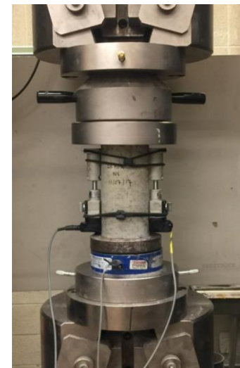
Figure 3.2. The Stiffness Damage Test (SDT), A– Stiffness Damage Index, SDI & Modulus of Elasticity, ME, B – SDT Setup (Sanchez et al. 2016)
