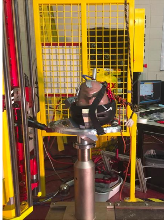
Figure 2. The Monorail Drop Rig with the helmeted (black) Hybrid III headform supported by the halo carriage. A 45° steel anvil is covered with blue sandpaper (coefficient of friction =0.5).
