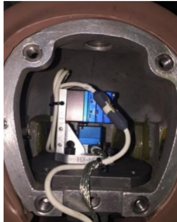
Figure 4. The tri-axial accelerometers with the three angular rate sensors located at the centre of gravity of the headform.
