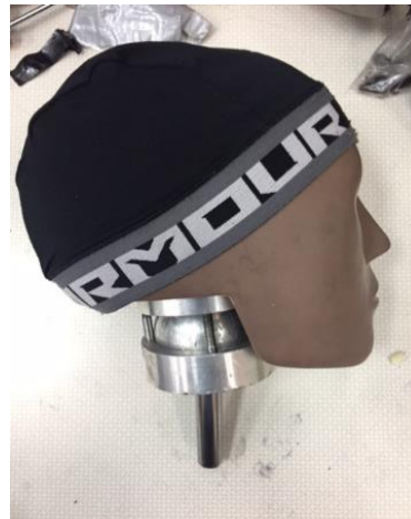
Figure 3. The male 50 th percentile Hybrid III headform with the release attachment containing three aluminum pieces (neck).
