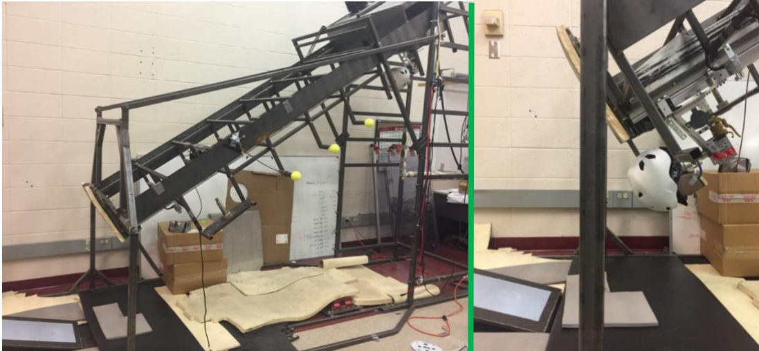
Figure 1. The angular launched impactor (ALI) angled at 30^\circ with the helmeted (white) Hybrid III headform located at the top (left image) and bottom (right image) of the system. A 15^\circ steel impact surface (anvil), covered with blue sandpaper (coefficient of friction =0.5), is located at the ending path of the system.
