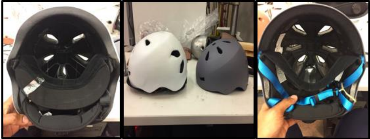
Figure 6. Center image displays the exterior shells of the PVC shell-PU liner helmet (left) and the ABS shell-EPS liner (right). The far left and far right images display the interior design of the PU liner with the comfort foams, and EPS liner with the comfort foams, respectively.
