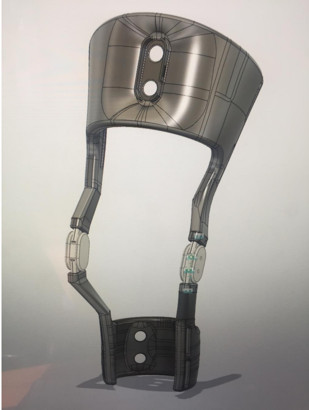
Figure 26 - Computer assisted-design of Prototype 2. The EMG sensor case is merged with the brace cuffs.
