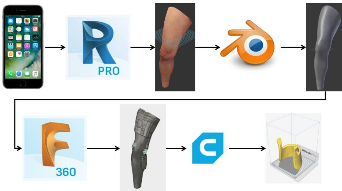
Figure 2 – Workflow. A smartphone was used for the data collection. Recap receives the data as input then outputs the cropped mesh to Blender. Blender further processes the mesh and outputs to Fusion 360. Fusion 360 outputs the custom brace design to Cura. The 3D printer instructions are generated by Cura.
