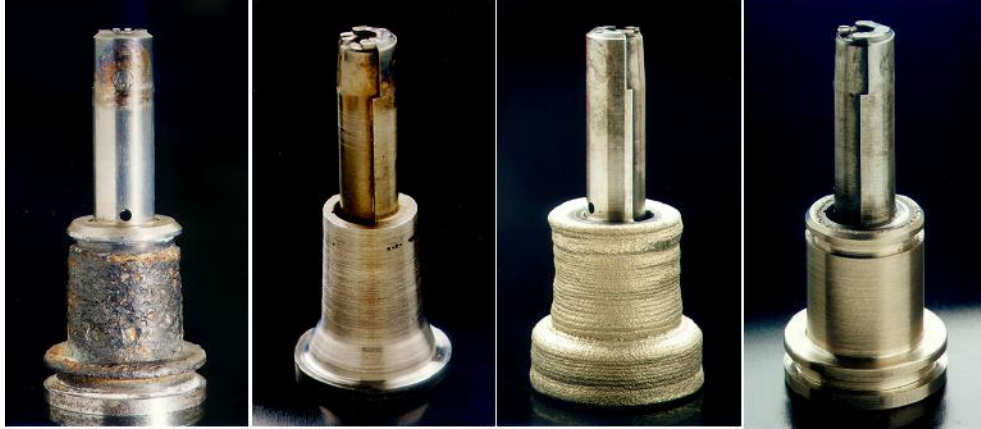
Figure 2.1: Laser beam cladding process used in industry [46]. The eroded part is machined down prior to the laser cladding process. The last step is the milling of the repair down to the original dimensions and tolerances.
