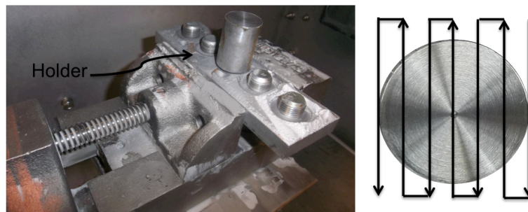
Figure 4.40: Set-up for the adhesion test during spray and spraying pattern (carbon fibre plates omitted in figure).
