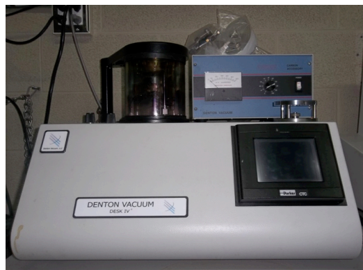
Figure 4.37: Gold sputtering equipment.
