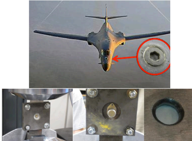
Figure 2.36: Skin panel repair using the cold gas dynamic spray process [125].
