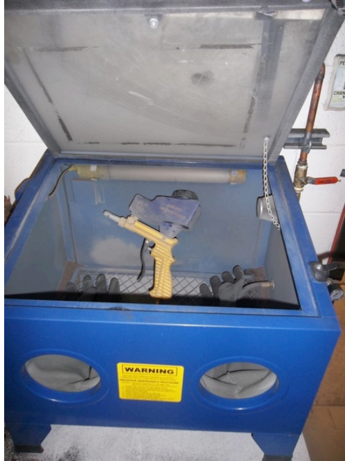
Figure 4.13: Grit blasting unit.
