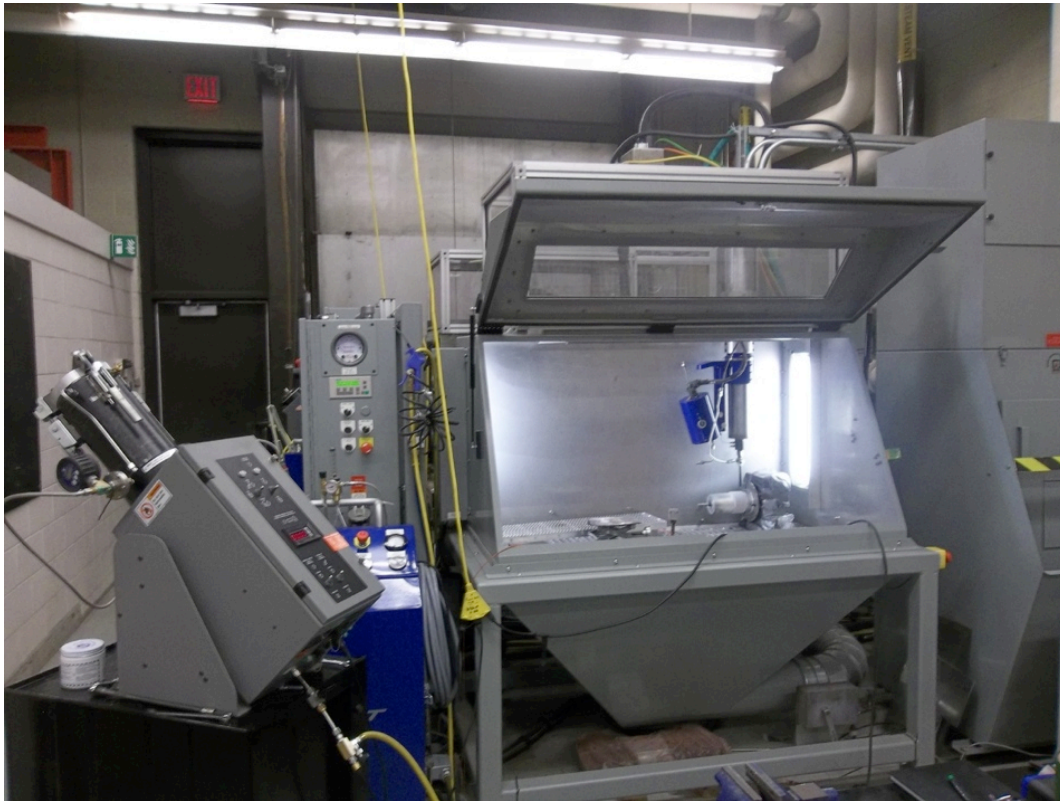
Figure 4.23: CGDS system overview (Centerline (Windsor) Ltd. SST-EP system).
