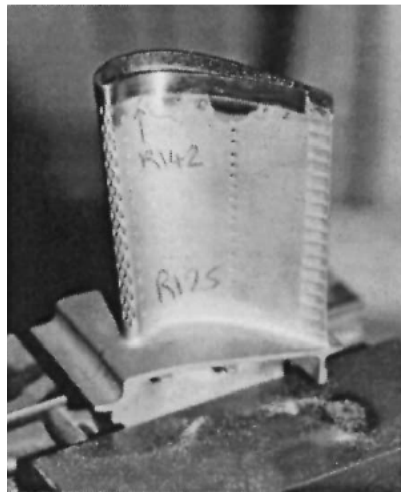
Figure 2.2: Turbine blade tip formed by laser cladding process [43].
