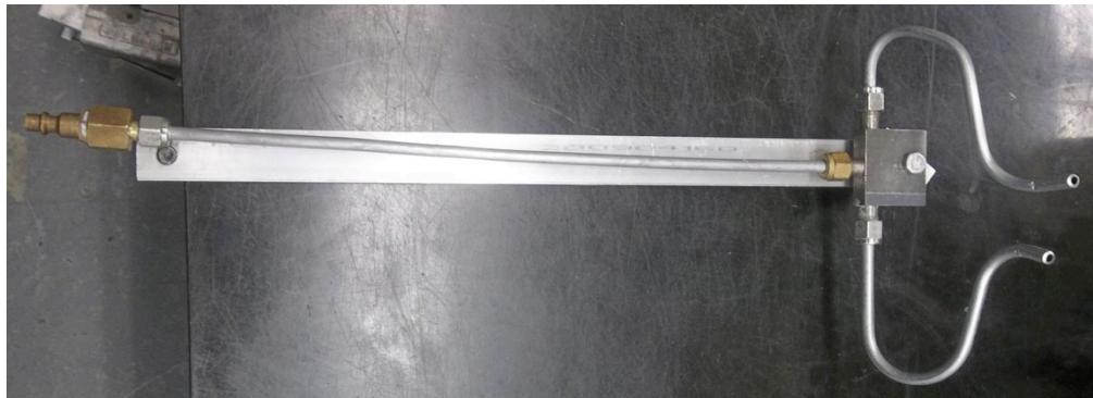
Figure 4.20: Aluminum tubing used to conduct air to the substrate surface for cooling purposes.
