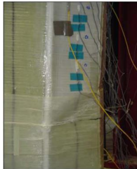
Local buckling failure specimen P3-
