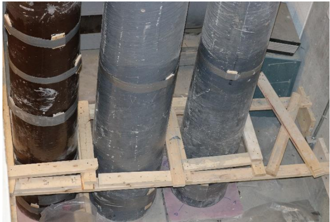
Lumber to secure the bottom of the specimens
