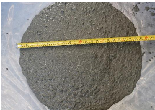
a. Slump flow for towers
