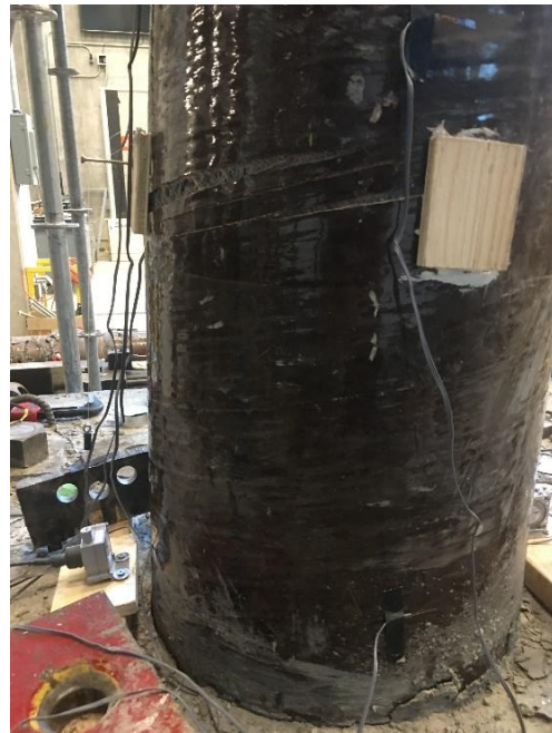
(b) GFRP rupture
