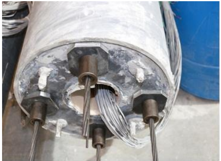
(b) Octagon plate with steel tendons installed
