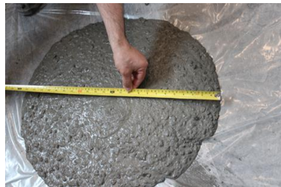
b. Slump flow for foundation
