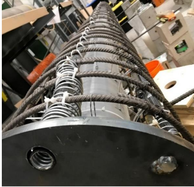
Figure 3.11. Galvanized wire wrapped around the end of the conduit
