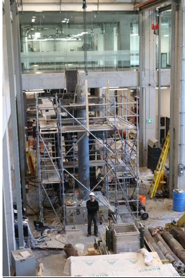
Figure 3.28. CFFT tower segment prior to testing
