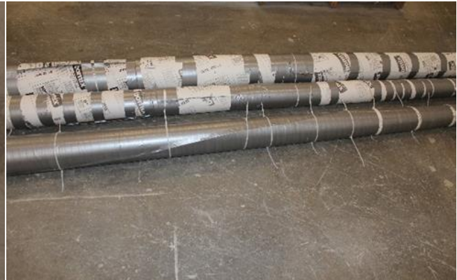
Stage 4. Wrapping sonotubes with duct tape
