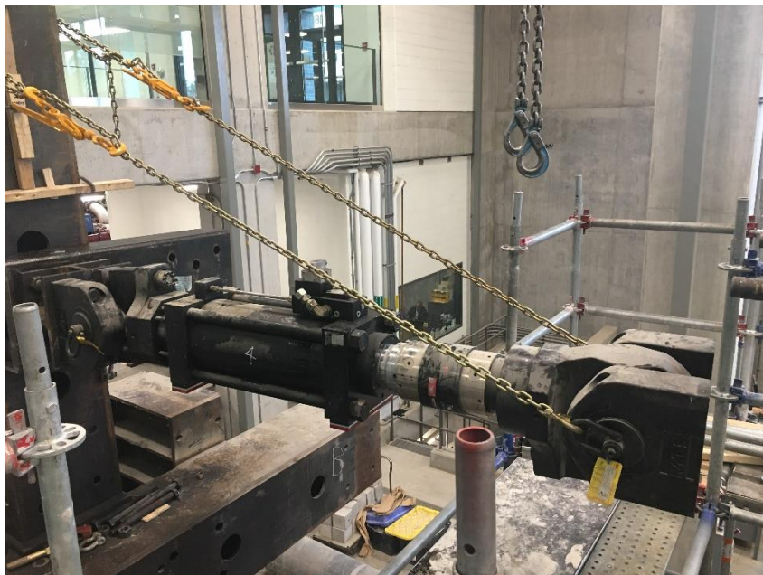
Figure 3.26. Steel chain with high safe workload capacity to support the actuator
