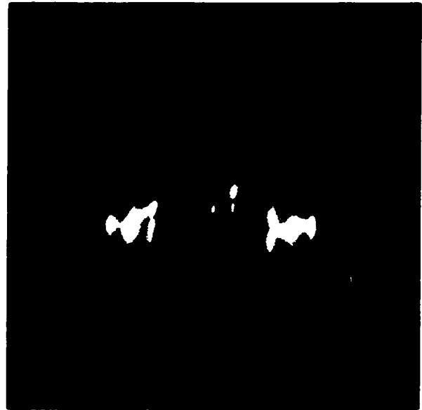
Figure 42. (2×4) GaAs (001) surface reconstruction, RHEED pattern of the [110] (i.e. e-beam along the [\bar{1}10] ). Compare to Figure 36.
