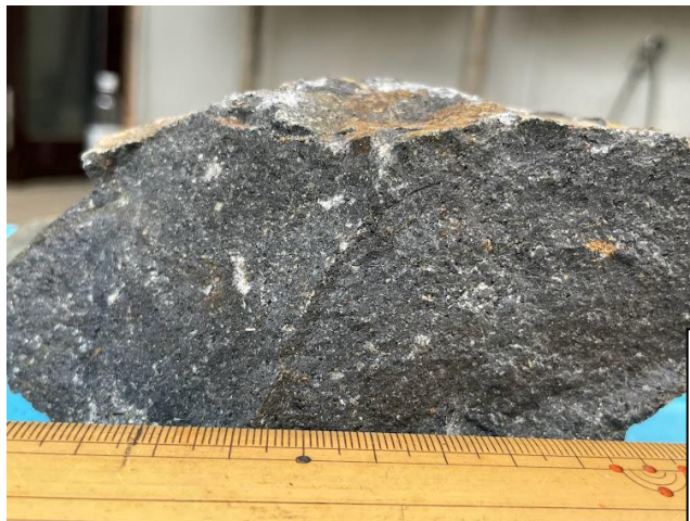
Porphyritic texture, outlining corroded bronze yellow mineral (<1mm)
