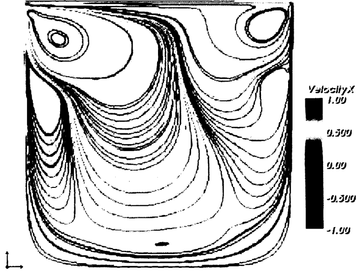
Figure 11: Streamlines colored by the x-velocity, Str = 1 , Re = 8000 , ( Wo = 112.07 ), t = 14 , U(x, 1, t) = \cos(\frac{2\pi t}{T})
