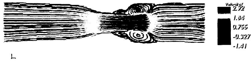
Figure 107: Streamlines colored by the x-velocity, Str = 0.5 , Re = 400 , ( Wo = 17.72 ), t = 12
