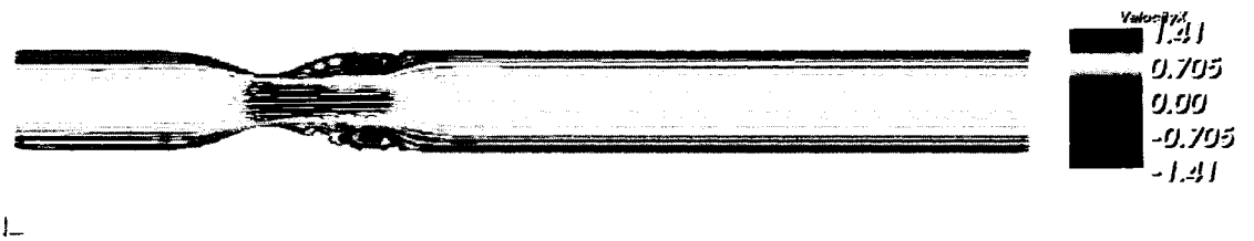
Figure 118: Streamlines colored by the x-velocity, Str = 1 , Re = 400 , ( Wo = 25.05 ), t = 6
