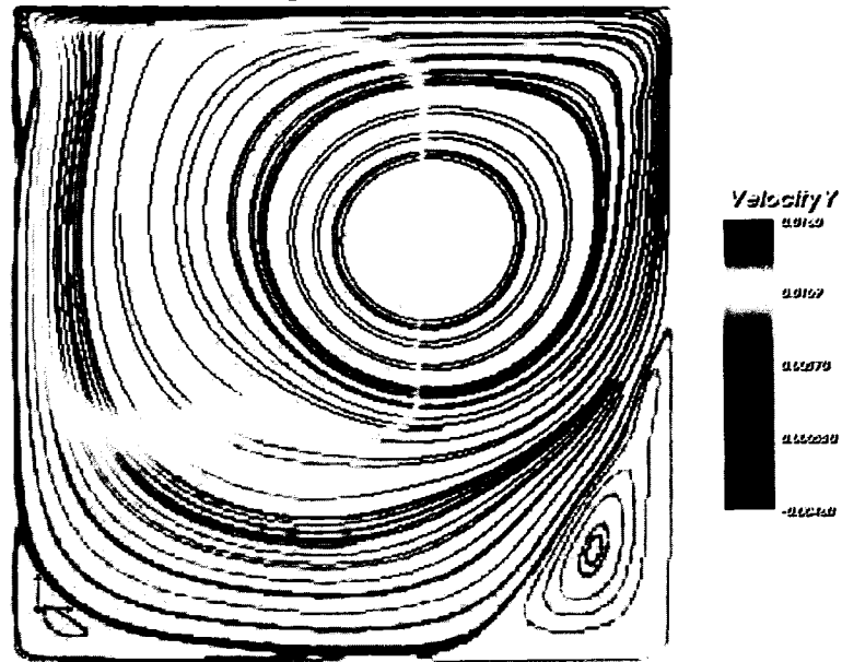
Figure 43: Streamlines colored by the y-velocity, Str = 1 , Re = 5000 , ( Wo = 88.6 ), t = 6 + \frac{T}{2} , U(x, 1, t) = (\max(\cos(\frac{2\pi t}{T}), 0), 0)
