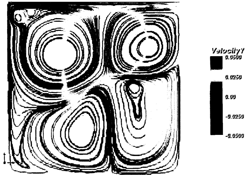
Figure 33: Streamlines colored by the y-velocity, Str = 0.1 , Re = 8000 , ( Wo = 35.44 ), t = 190 + \frac{T}{2} , U(x, 1, t) = \cos(\frac{2\pi t}{T})
