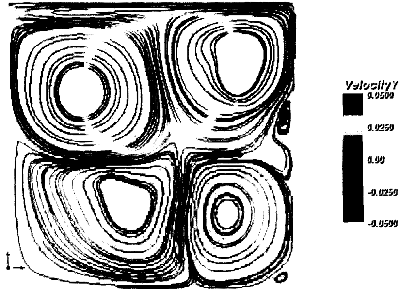
Figure 31: Streamlines colored by the y-velocity, Str = 0.1 , Re = 8000 , ( Wo = 35.44 ), t = 190 , U(x, 1, t) = \cos(\frac{2\pi t}{T})
