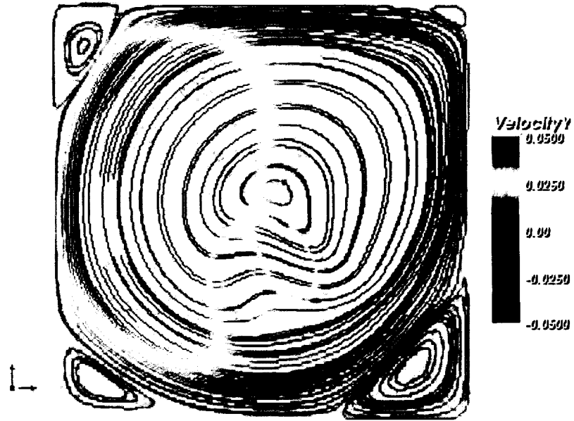
Figure 57: Streamlines colored by the y-velocity, Str = 0.1 , Re = 5000 , ( Wo = 28.01 ), t = 190 + \frac{T}{2} , U(x, 1, t) = (\max(\cos(\frac{2\pi t}{T}), 0), 0)
