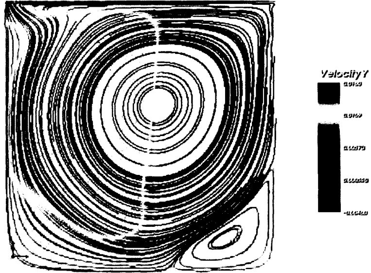
Figure 45: Streamlines colored by the y-velocity, Str = 1 , Re = 8000 , Wo = (112.07) , t = 30 , U(x, 1, t) = (\max(\cos(\frac{2\pi t}{T}), 0), 0)
