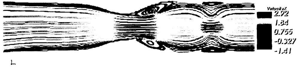
Figure 80: Streamlines colored by the x-velocity, Str = 1 , Re = 400 , ( Wo = 25.05 ), t = 8
