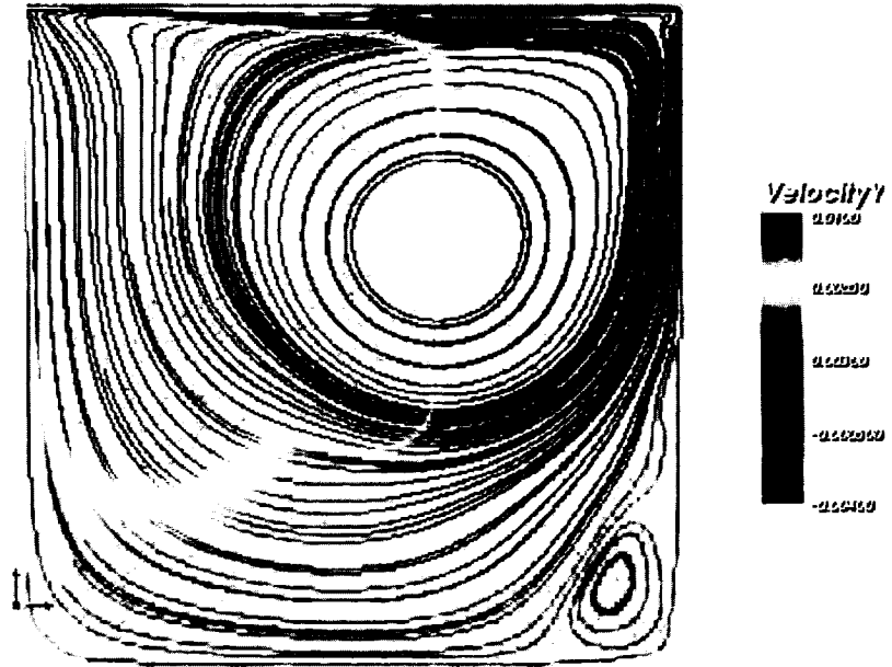
Figure 41: Streamlines colored by the y-velocity, Str = 1 , Re = 5000 , ( Wo = 88.6 ), t = 6 , U(x, 1, t) = (\max(\cos(\frac{2\pi t}{T}), 0), 0)
