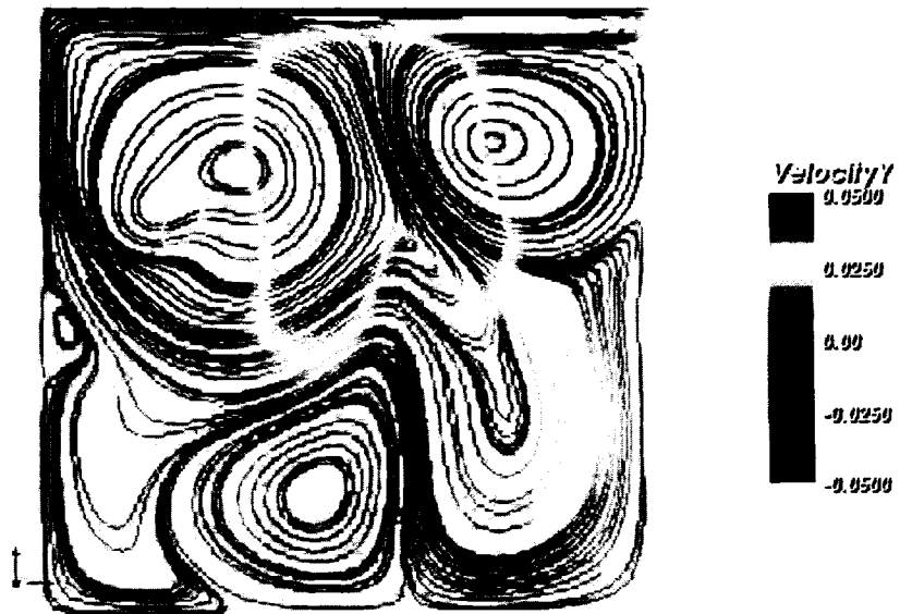
Figure 33: Streamlines colored by the y-velocity, Str = 0.1 , Re = 8000 , ( Wo = 35.44 ), t = 190 + \frac{T}{2} , U(x, 1, t) = \cos(\frac{2\pi t}{T})
