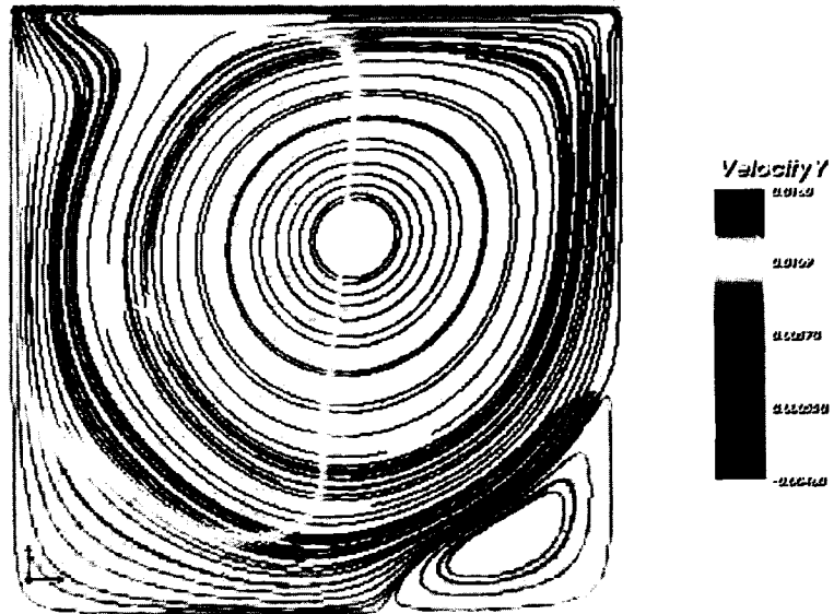
Figure 45: Streamlines colored by the y-velocity, Str = 1 , Re = 8000 , Wo = (112.07) , t = 30 , U(x, 1, t) = (\max(\cos(\frac{2\pi t}{T}), 0), 0)
