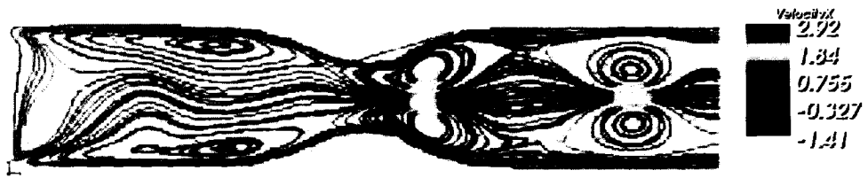
Figure 81: Streamlines colored by the x-velocity, Str = 1 , Re = 400 , ( Wo = 25.05 ), t = 8 + \frac{T}{4}
