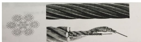
Figure 2-3: Strand rope cross-section and side view [14].
