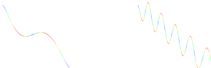
Figure 3-6: 3 rd , 19 th mode shape of uniform property cable
