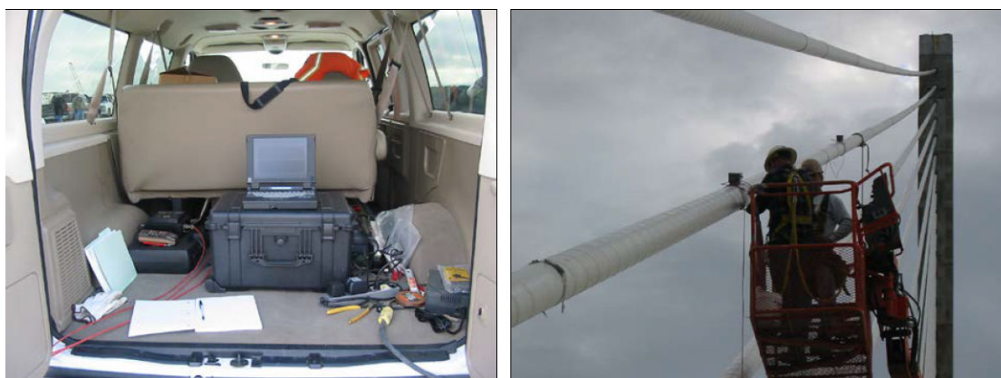
Figure 4-31: The data acquisition system (left) and mounting accelerometers on a stay cable (right) [78]
