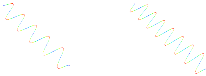
Figure 3-7: 20 th , 29 th mode shape of uniform property stay-cable
