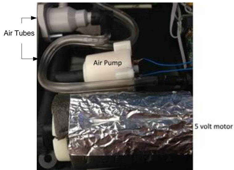
Figure 17 Air Tubes, Air Pump and Motor
