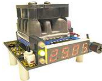
Figure 117: Butterfly socket Thorlabs LM14S2 (a), temperature controller WTC3243 (b)
