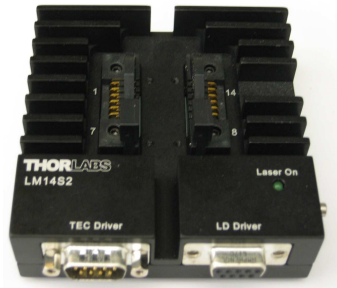
Figure 117: Butterfly socket Thorlabs LM14S2 (a), temperature controller WTC3243 (b)
