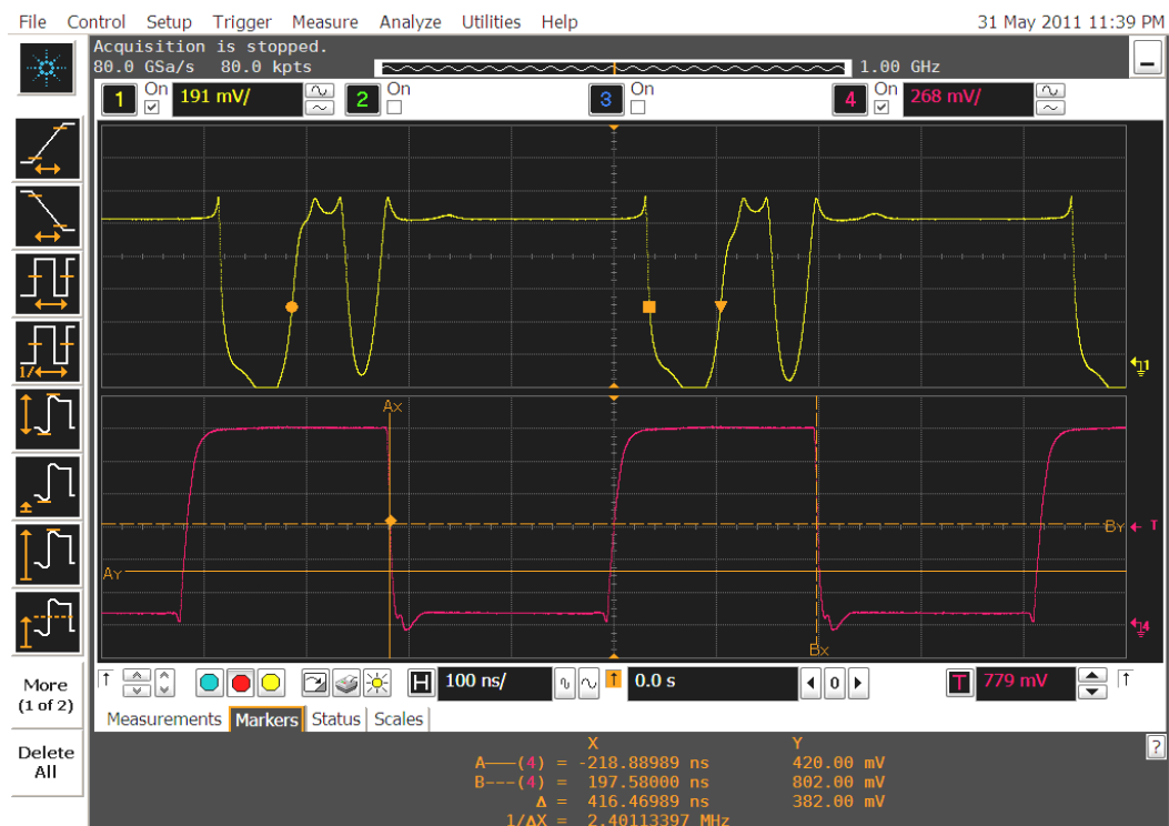
Figure 124: Distorted SOA response signal (upper) at 2.4 MHz modulating signal (lower)
