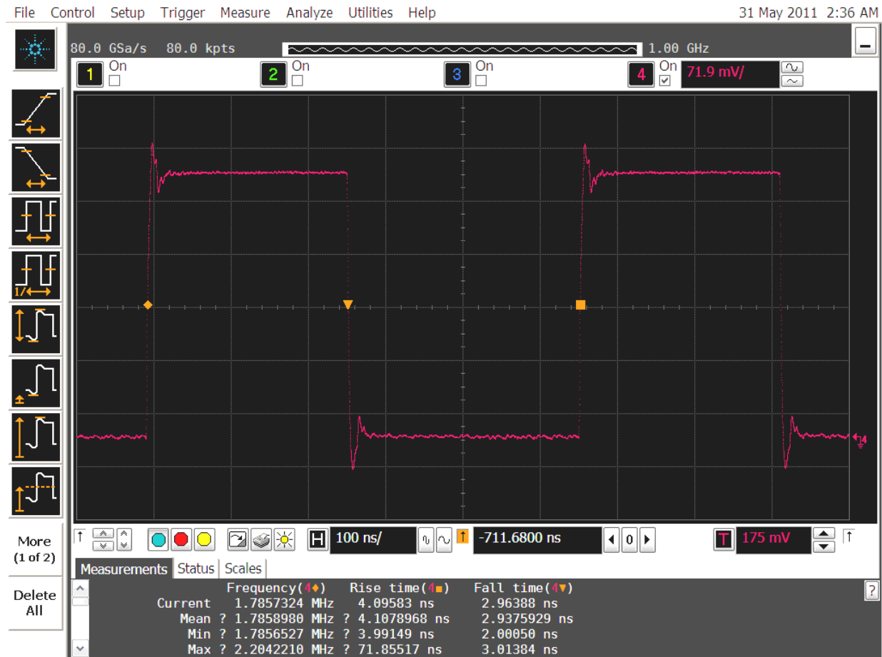
Figure 135: Speed benchmark of the FPGA-based controller
