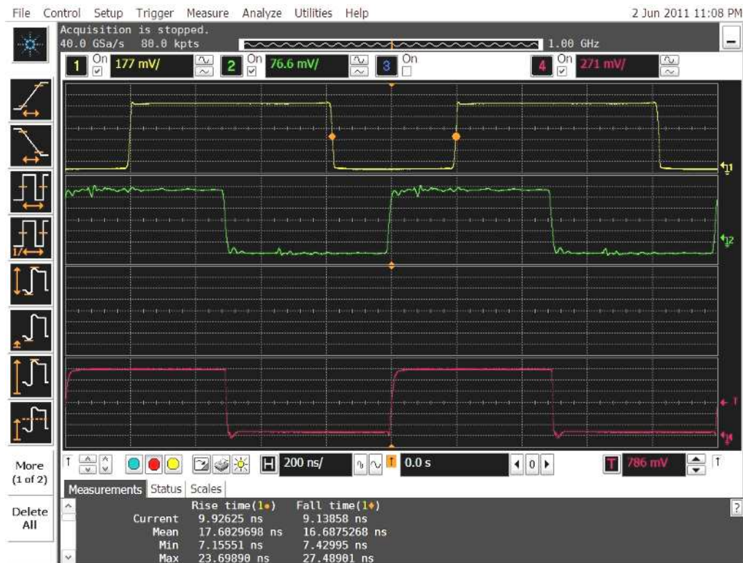
Figure 126: Comparison of the 1 MHz modulating signal (bottom), driver signal (middle) and SOA response signal (top).
