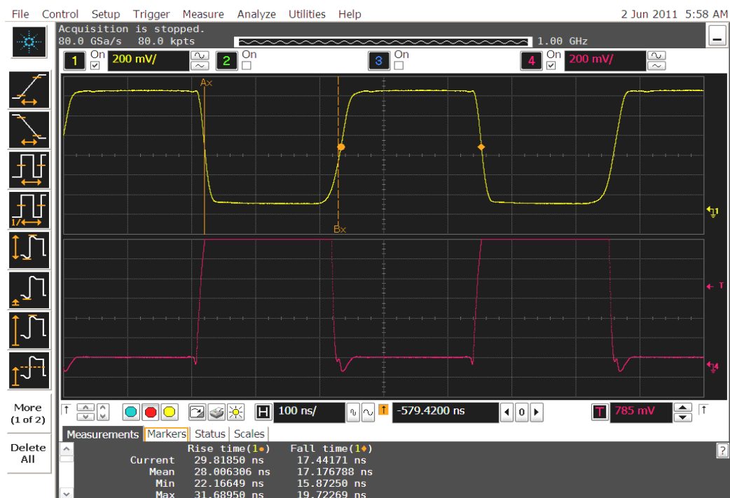
Figure 123: SOA response signal (upper) and 2.3 MHz modulating signal (lower)
