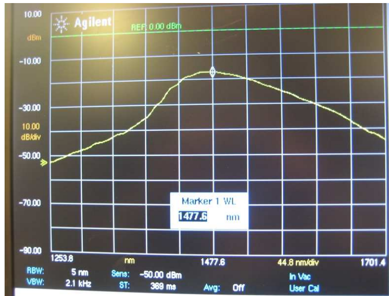
Figure 158; Spectrum of the optical signal emitted by SOA OPB1010NCFA when supply current is 100 mA. (No input optical power present).
