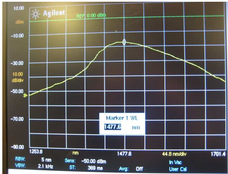
Figure 113: Spectrum of the optical signal emitted by Kamelian SOA at 100 mA with no input optical power present.
