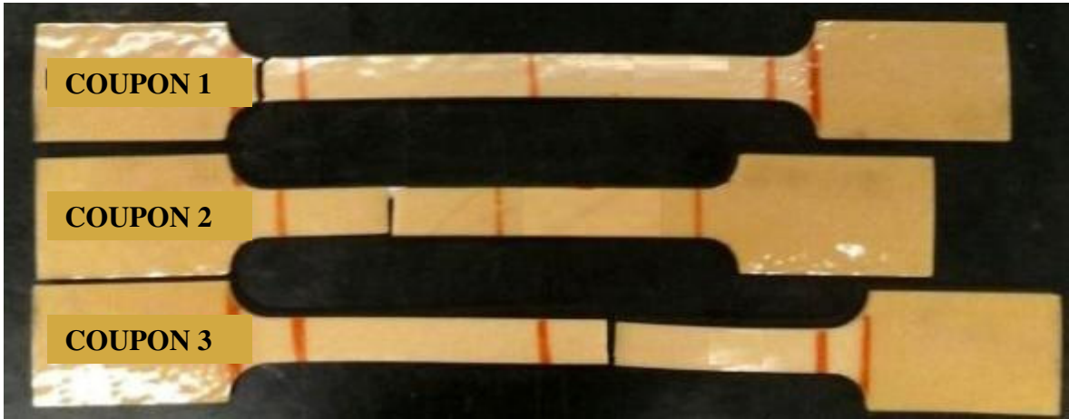
Figure 2.19: Polyurea Coupons after Rupture
