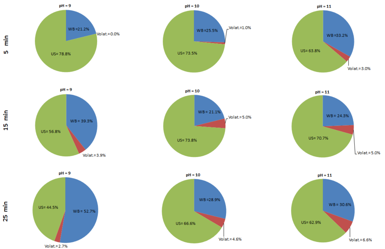
Figure 4.5 Percentage of TAN removal by non-thermal (US), thermal (WB), and volatilization (Volat.) at different pH and time duration
