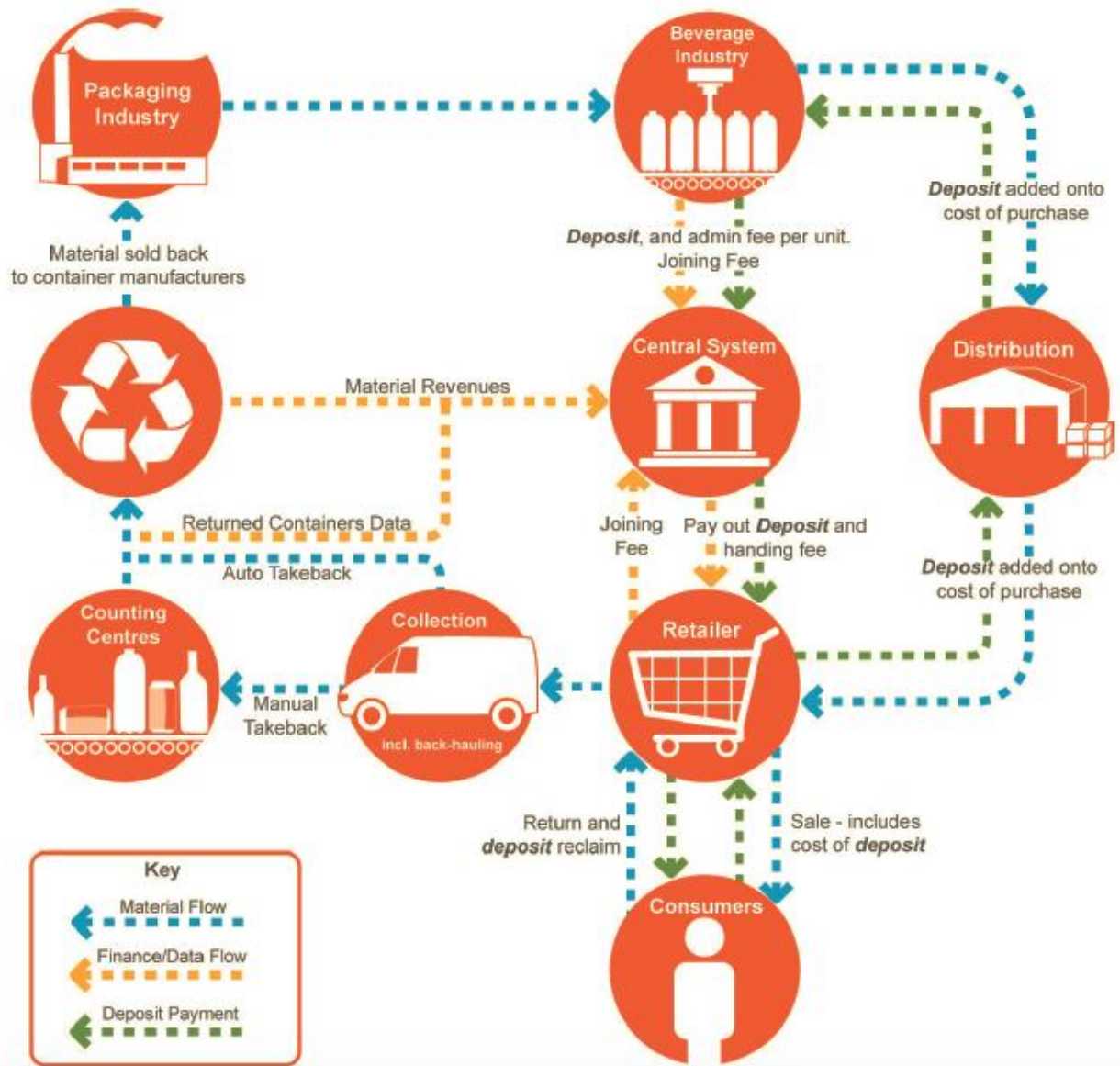
Figure 2: The general material and financial flows of a return-to-retail DRS, developed by Eunomia (Hogg, et al., 2017).
