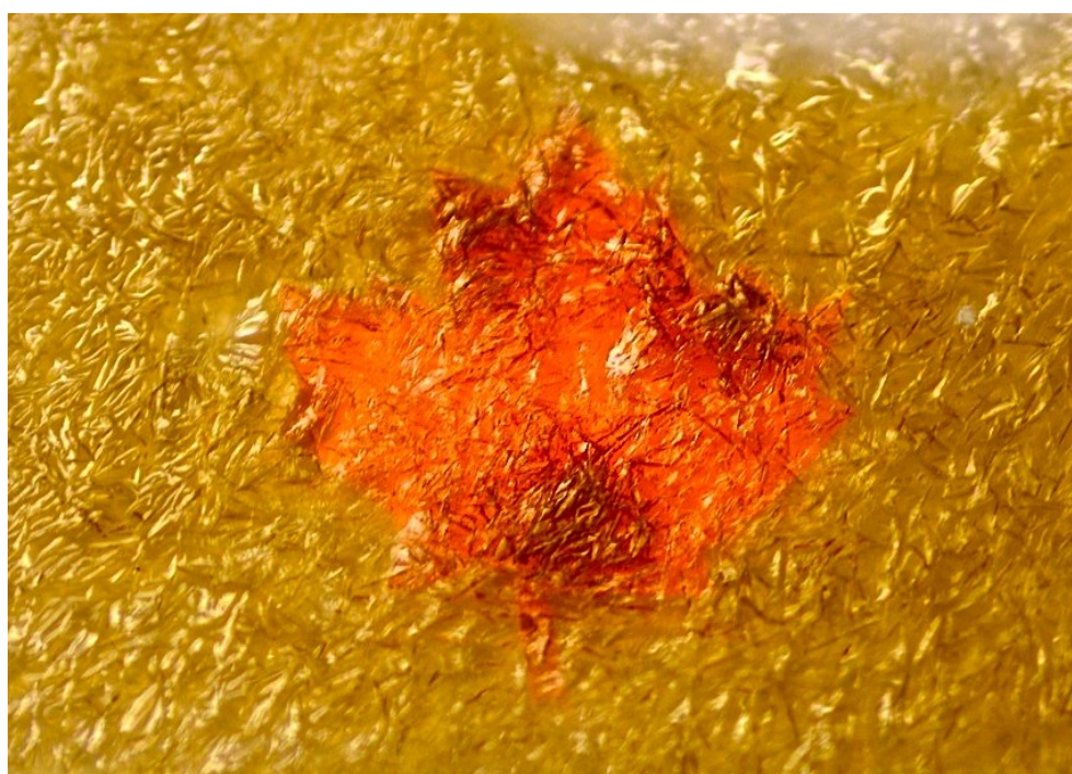
Figure 4.9: The red leaf represents the area where AuNRs have been aligned upon exposure to 690 nm light. The maple leaf is 11.4 mm wide and the film thickness is 0.58 mm.
