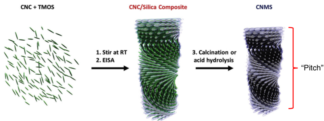
Figure 6.5: Diagram exemplifying the synthesis of chiral-nematic mesoporous silica materials. Reproduced with permission from ref.[15]. Copyright (2017) Wiley.
