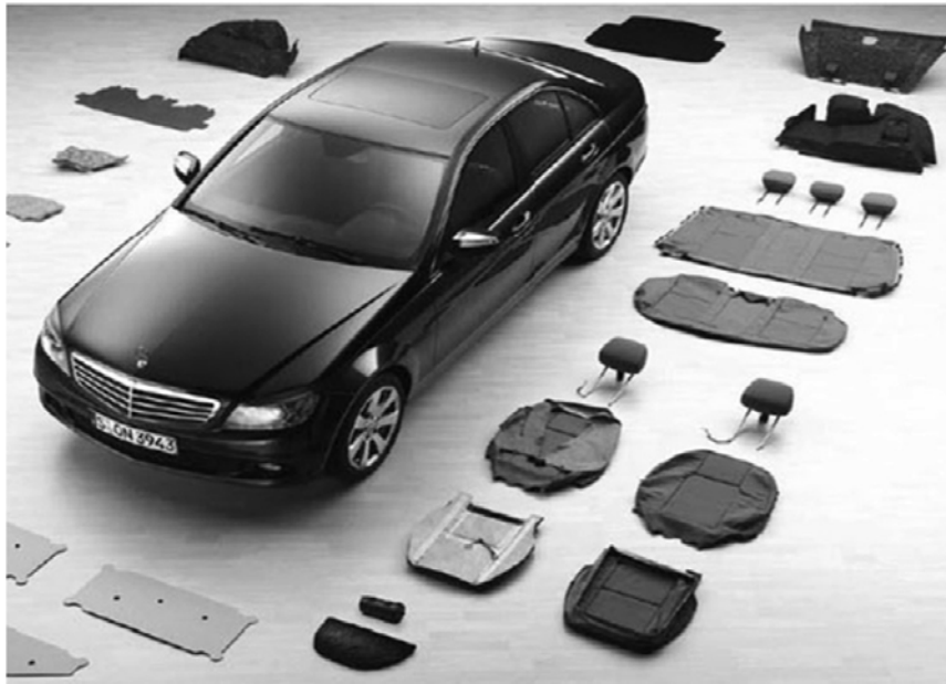
Figure 1.6. Components featuring PMFRC parts used in a production car [8]
