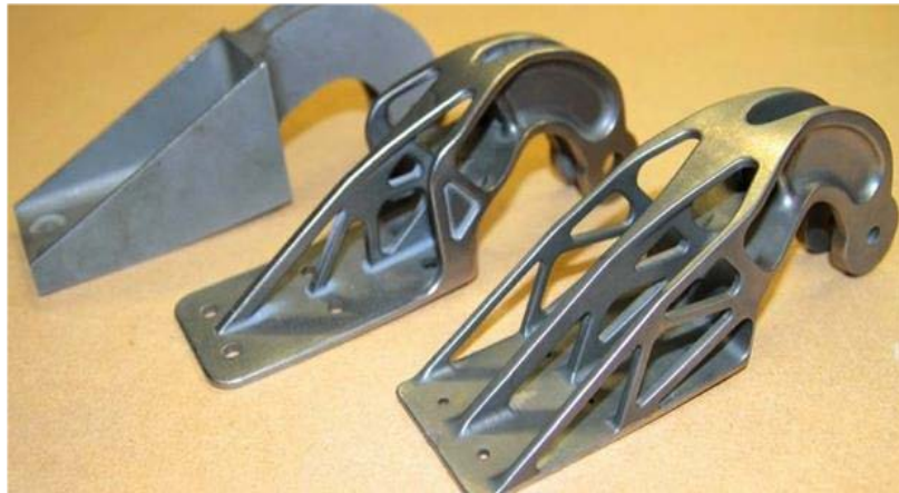
Figure 4.7. Metal AM parts 3D printed for European Space Agency [120]
