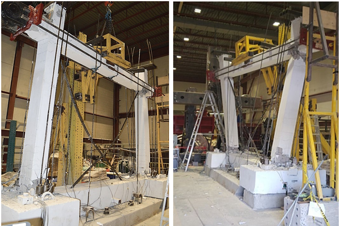
Figure 4-30 Test frame at the end of the test - PEC Arrangement 2
