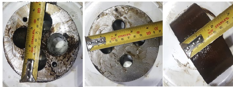
Anchor head front Anchor head back Anchor head side (b) Anchor head that can accommodate up to 4 strands
