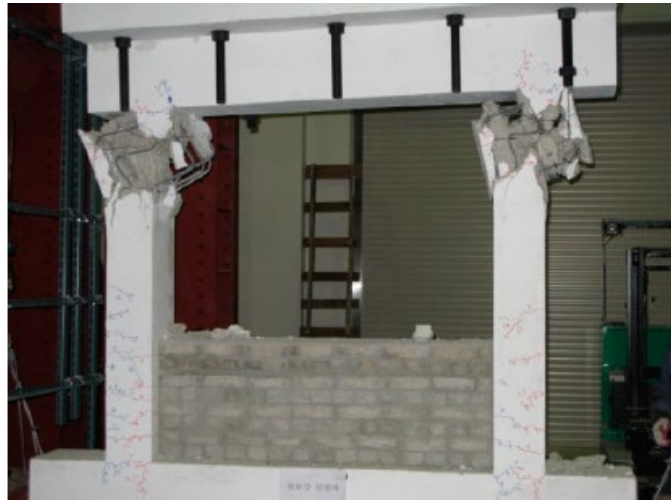
Figure 2-34 Failure of the columns at the end of the test (Lee 2015)
