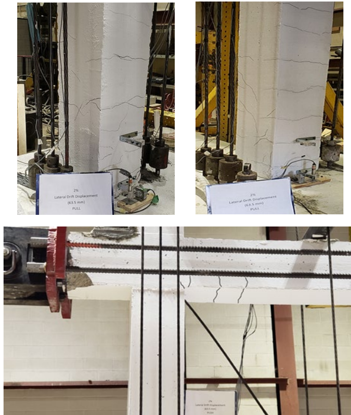
Figure III-2 Crack pattern during Test 1 after 2% drift cycles
