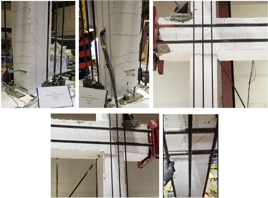
Figure III-3 Crack patterns at the end of 2.5% drift cycles
