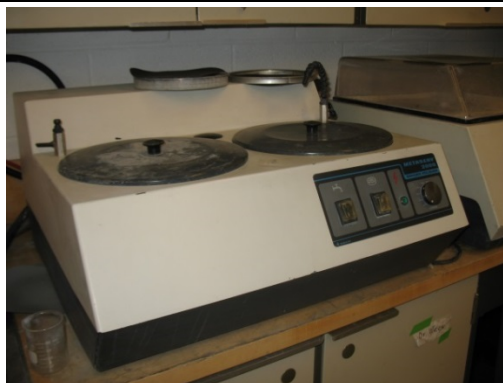
Figure 47. The Buehler Metaserv 2000 polishing apparatus used in this project
