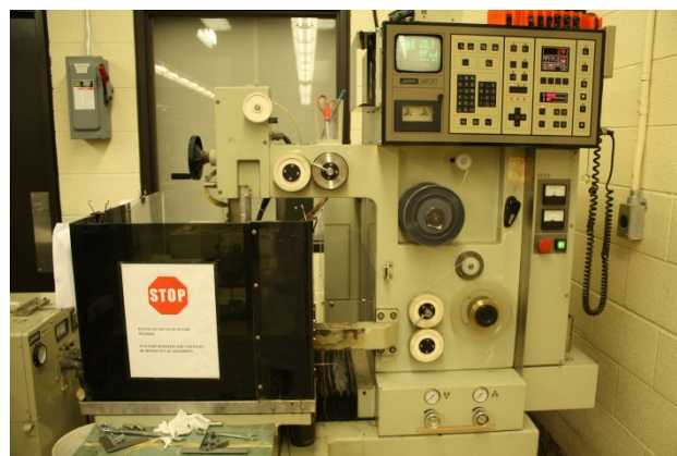
Figure 42. EDM (Electric discharge machining) at the Mechanical machine shop in the University of Ottawa.
