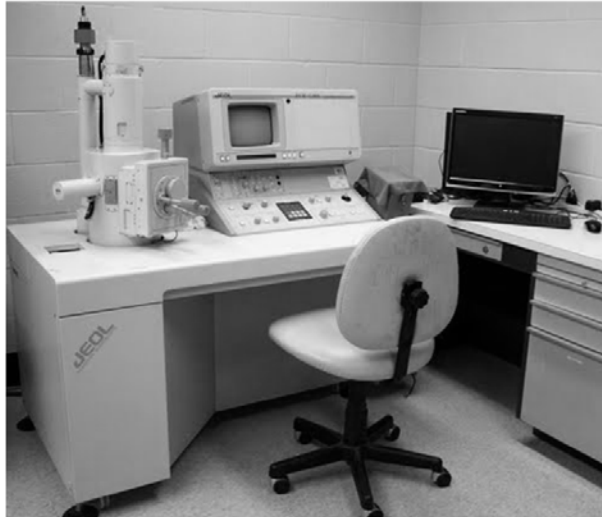
Figure 60. JEOL JSM-5300 Scanning Electron Microscope (SEM); Resolution: 10-20 nm, Magnification: high vacuum mode 15x-200,000x and low vacuum mode 15x-50,000x, Acceleration voltage: 0.5-30 kV, Specimen size: up to 76 mm in diameter.
