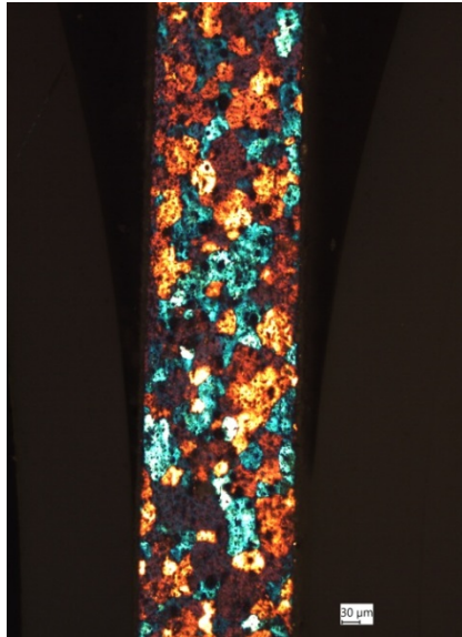
Figure 45. Optical micrograph of the cross section of a specimen annealed at 625°C for 2 hours.
