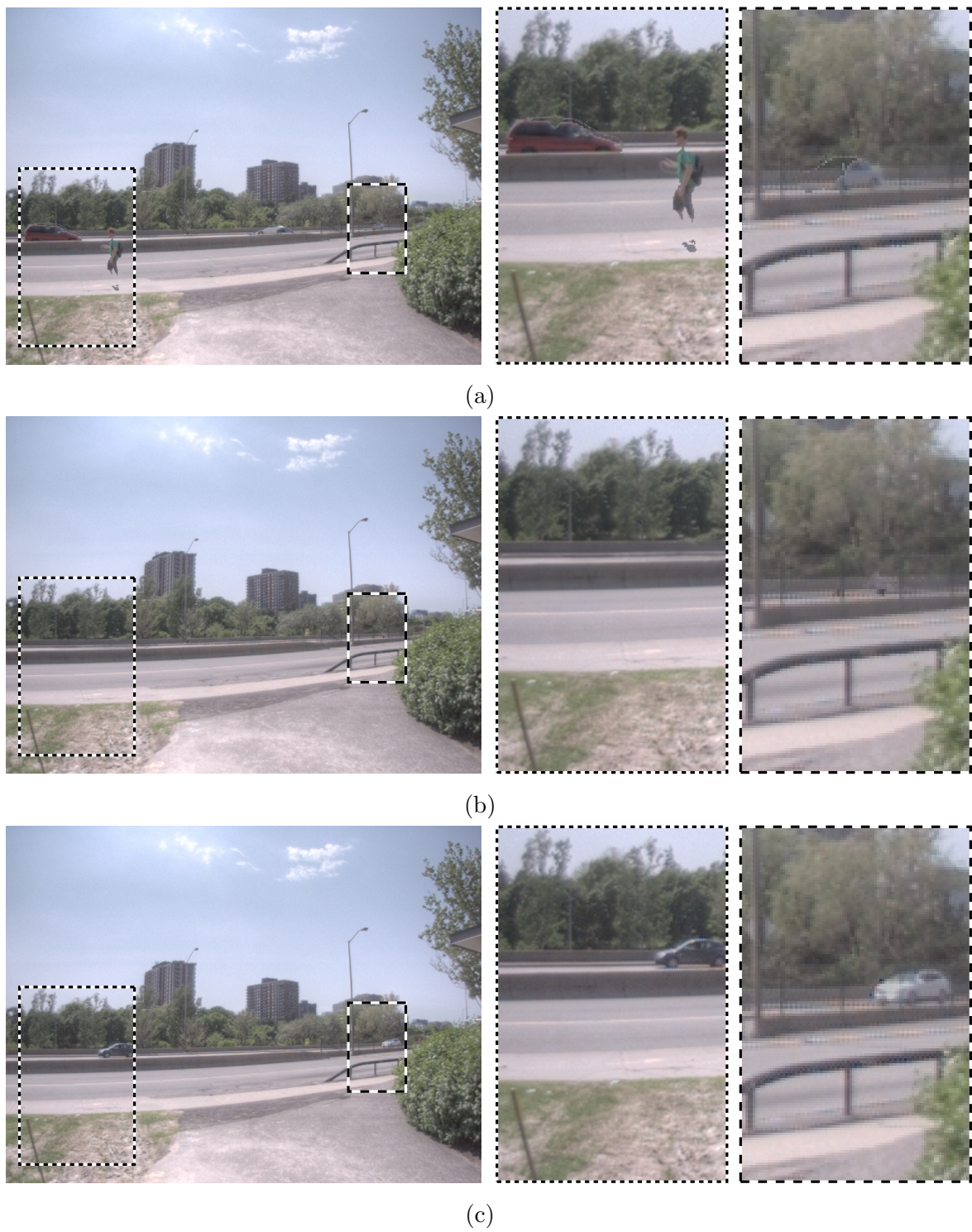
Figure 6.22: Alternate fluid motion fix options. a Pull replacements from best exposed image. b No fluid motion fix. c Pull replacements from best match for background.
