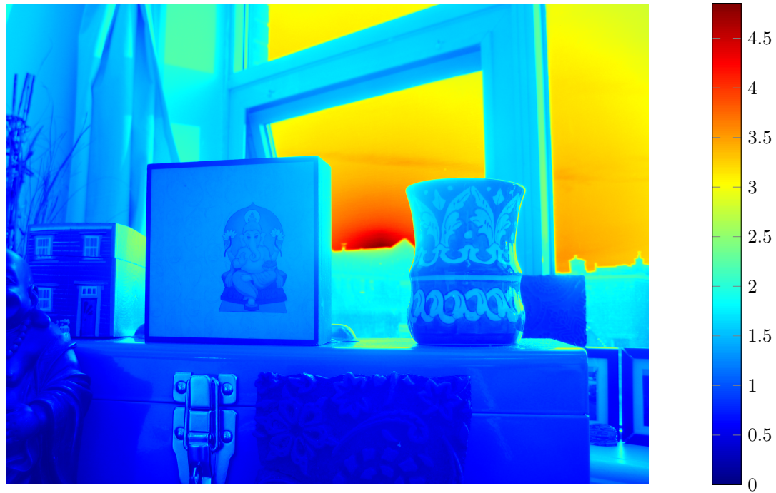
Figure 2.4: False-colour visualization of the intensity of an HDR image with approximately 77,000:1 dynamic range. The scale shows intensities in orders of magnitude or \log_{10} units relative to the darkest point in the scene.
