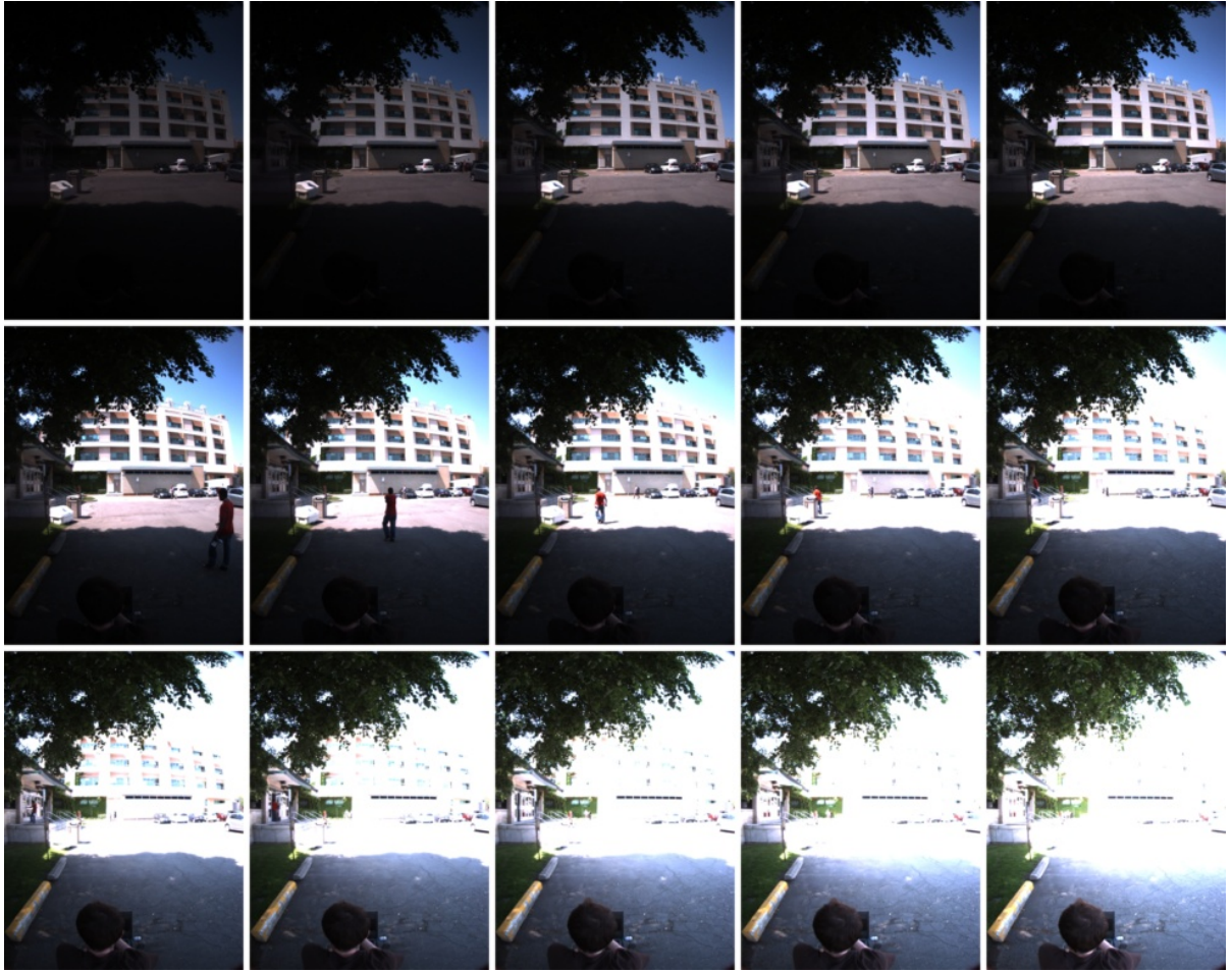
Figure 5.1: 15 of a 16-image sequence of exposure-bracketed images of the same scene displaying motion corruption. The scene is corrupted by multiple people walking through (discrete ghosts), as well as a large section of foliage blowing in the wind (fluid ghosting).
