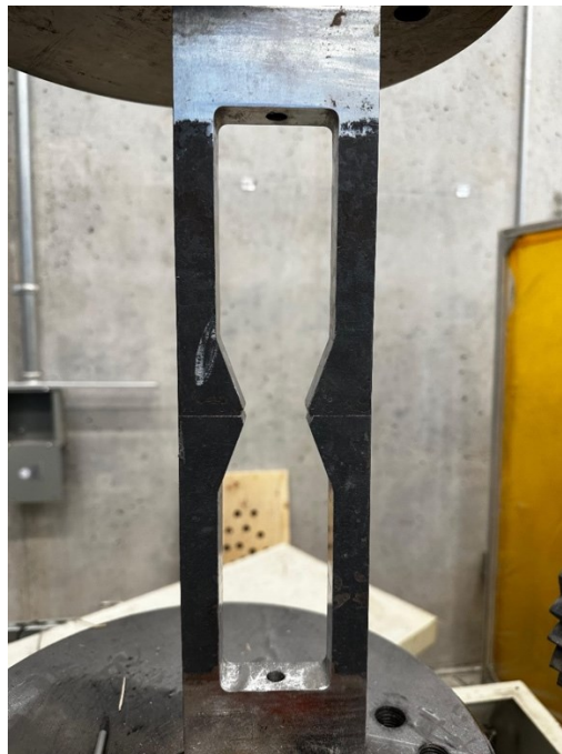
Figure 39: Alignment of U-shaped load application plates before tension tests
