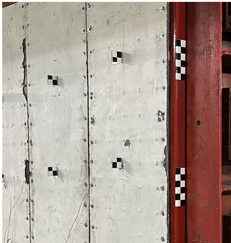
Figure 62: Checkerboard tape markings on wall specimens
