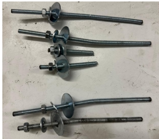
Figure 85: Threaded rods after failure
