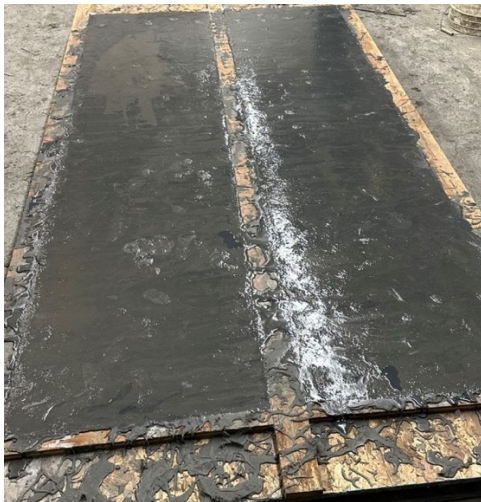
Figure 46: Specimens immediately after pouring and covered with wet burlap, four hours later
