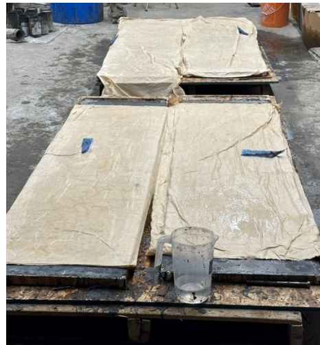
Figure 46: Specimens immediately after pouring and covered with wet burlap, four hours later
