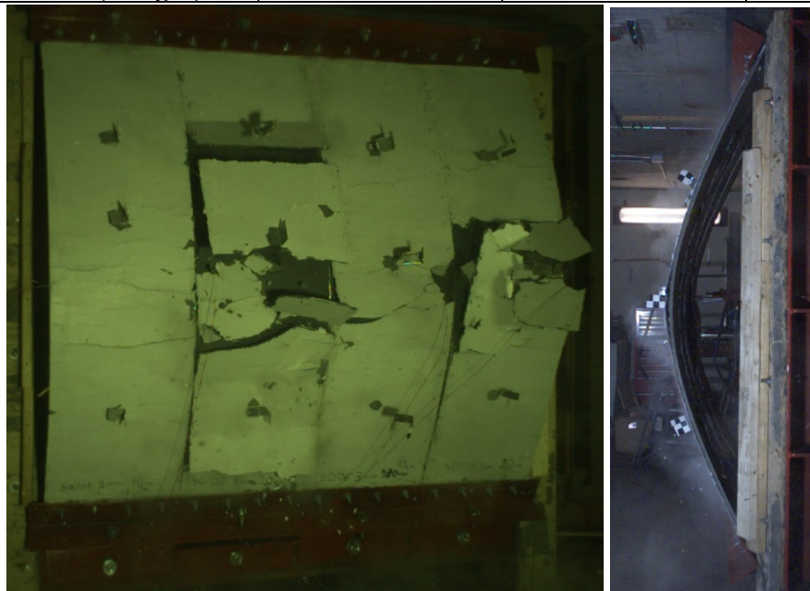
Figure 77: Set 2 shot #3 fragmentation at panels 2 and 4 (left), 309 mm additional deformation (right)
