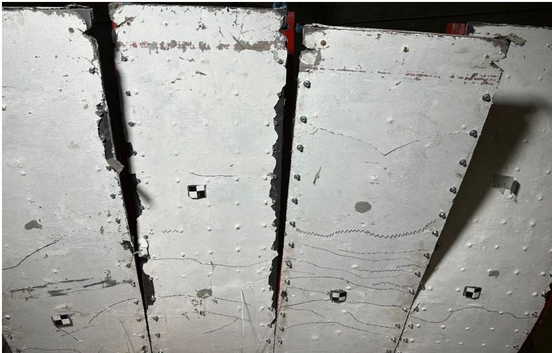
Figure 68: Set 1 specimens after failure, front side
