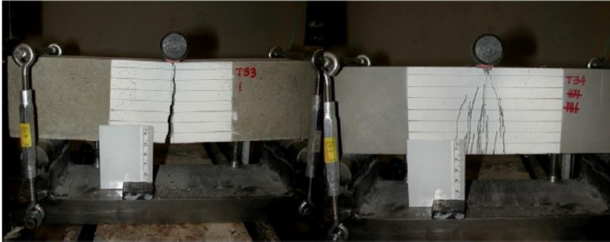
Figure 17: Impact performance of R/C vs R/ECC mix beams (Yang & Li, 2012)
