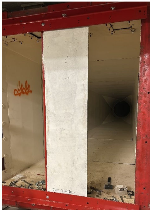
Figure 51: A single panel and an HSS member behind at its left-hand side
