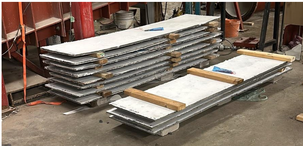
Figure 47: Panel specimens prior to installation on the shock tube for blast testing
