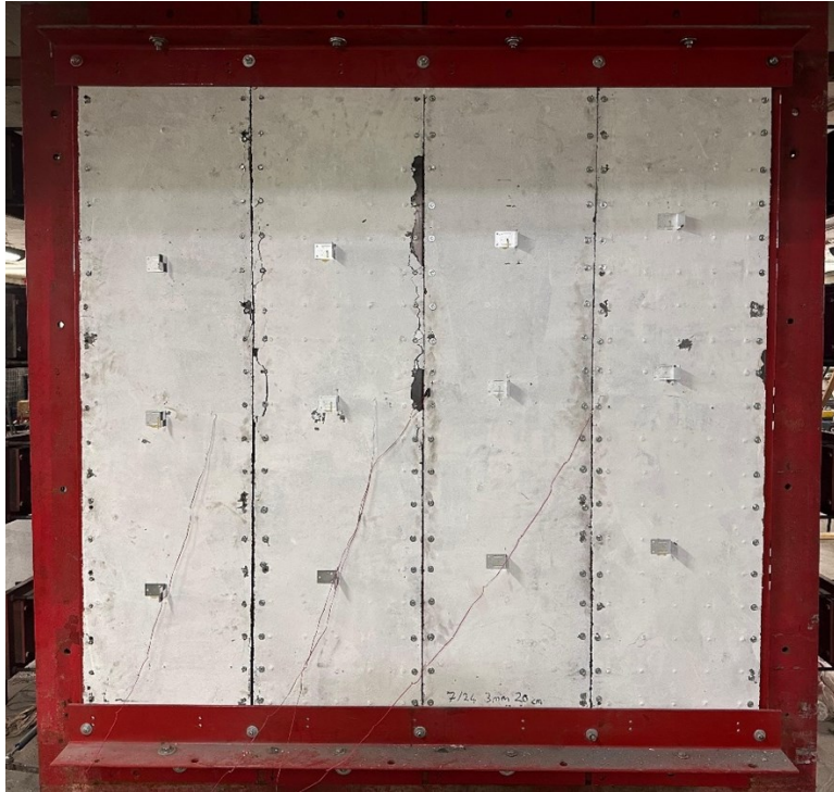
Figure 61: Displacement measurement locations on the panels
