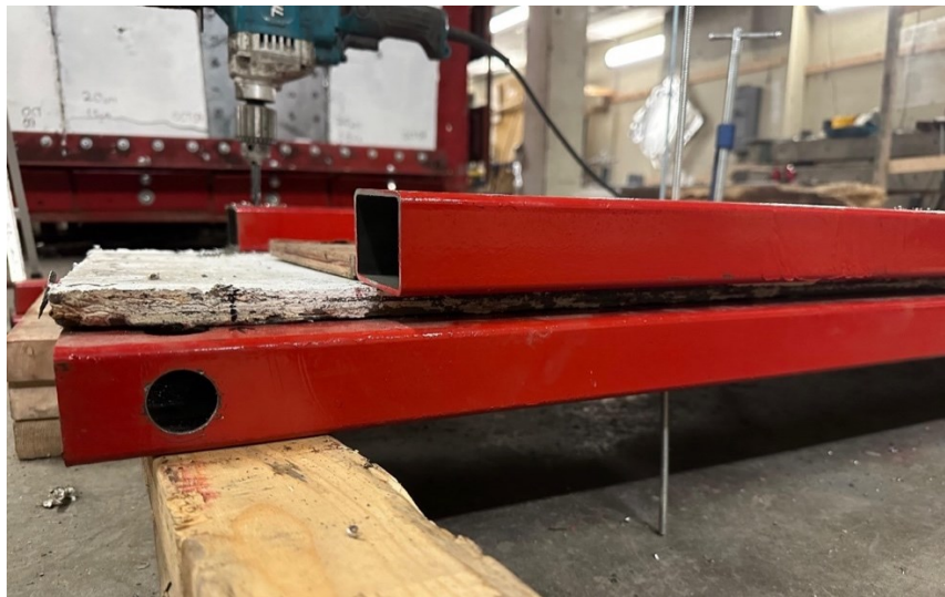
Figure 58: Set 4 specimens during preparation
