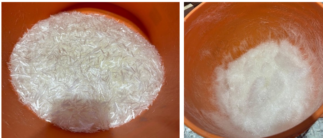
Figure 44: Fibres before (left) and after (right) air-tumbling
