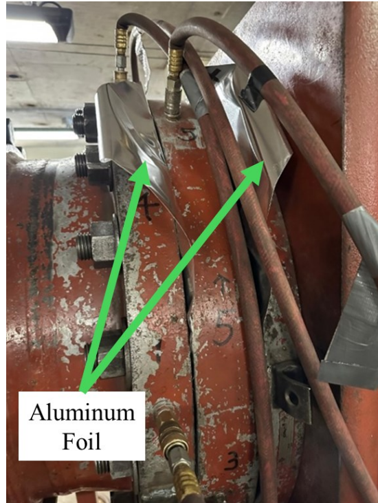
Figure 49: Aluminum sheets on either side of the diaphragm section
