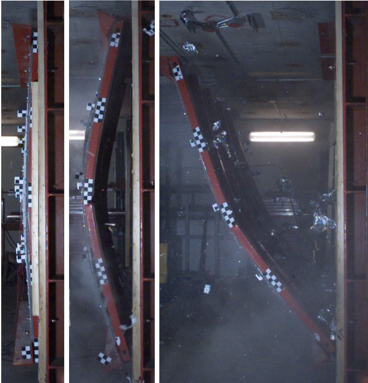
Figure 66: Set 1 specimens before and during shot #6
