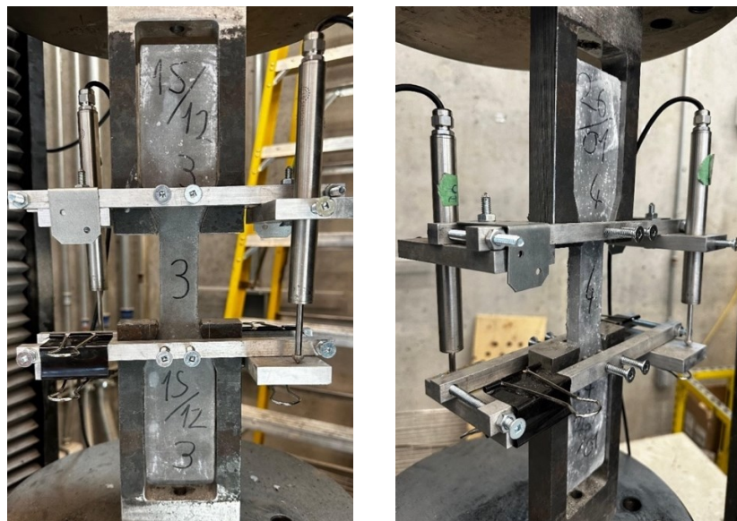
Figure 38: Direct tension test setup of ECC coupons, LVDTs on the right front and left behind
