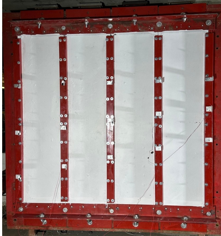
Figure 59: Set 4 wall specimens prior to testing
