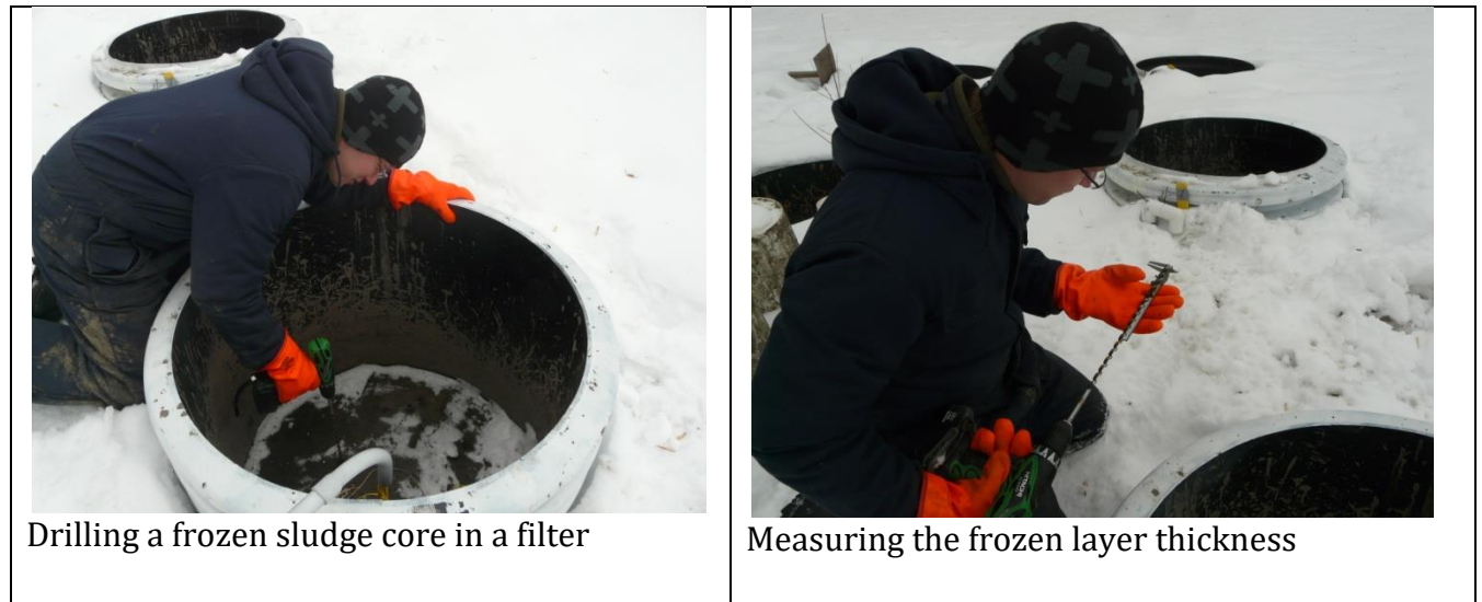
Figure 4-5. Photos of Measuring Frozen Sludge Layer Thickness
