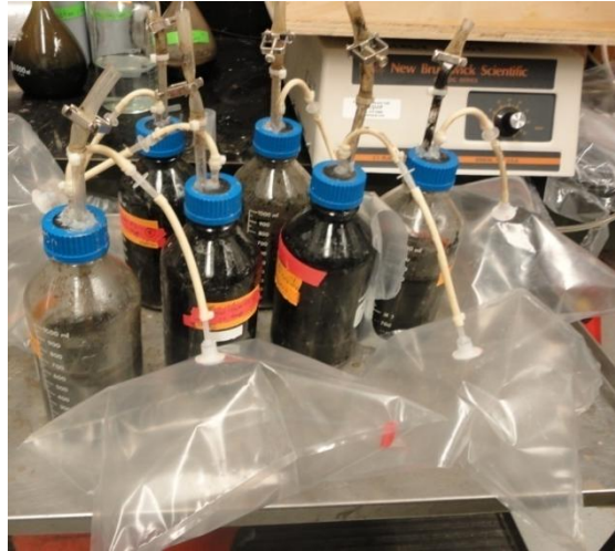
Figure A-4 Semi-continuous flow reactors
