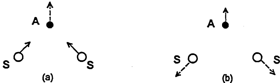
Figure 6.3: Normal modes of an adatom and bridge atoms.
