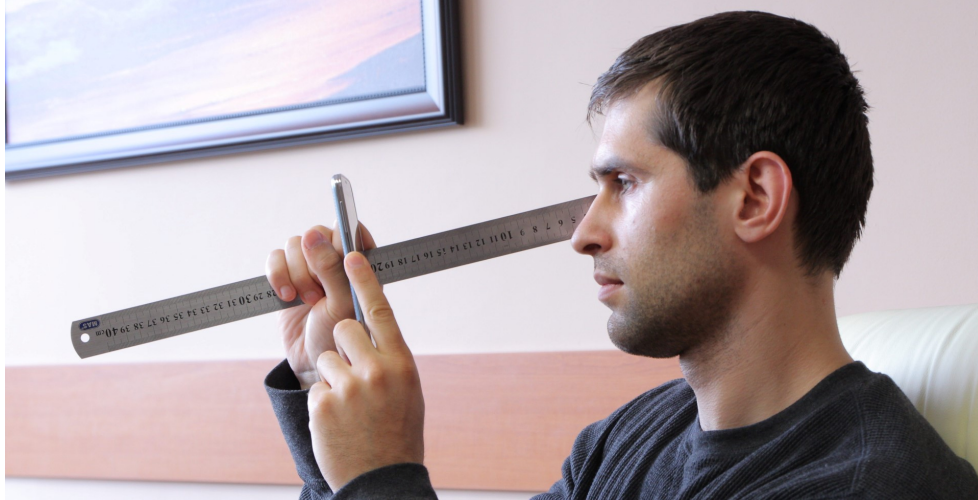
Figure 1.2: Average person starts noticing pixelization at around 7.8 inches in a 5-inch 1080p phone 7
