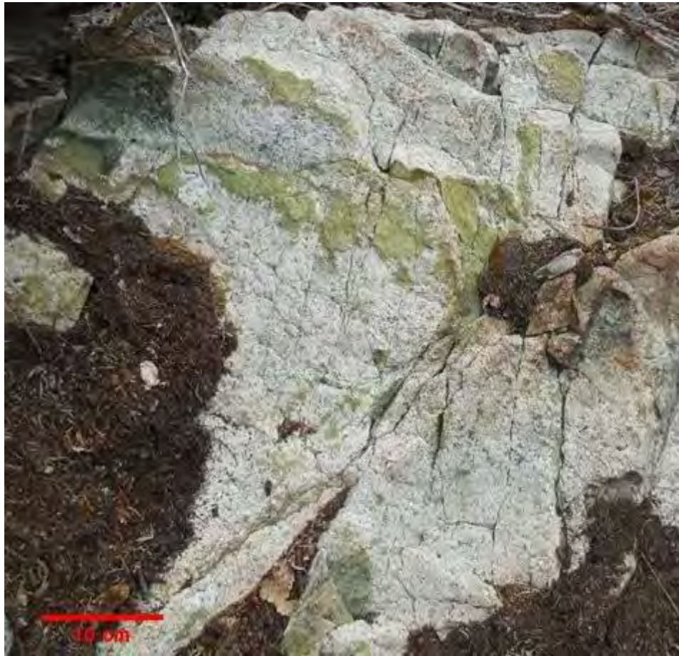
Figure 5. Outcrop at sample site GBR-39. Note the wide irregular epidote veining in leucocratic tonalite of the Granite Mountain batholith. Location: Easting 0555489 Northing 5826958 (NAD 83).
