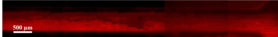
Figure 29. Fluorescence image of protein gradient formed using the Y-shaped channels in the microfluidic chip. Laminin is diluted with PBS to aid in the formation of a linear concentration profile. Laminin concentration increases from top to bottom.
