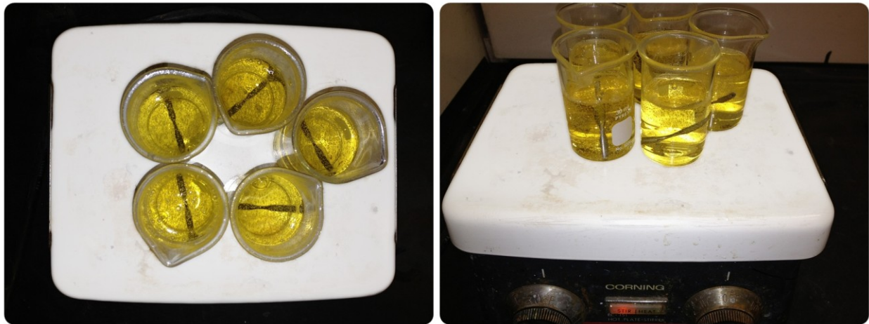
Figure 31. Beakers containing piranha solution and titanium samples on stirring plate at the end of oxidative nanopatterning process for 2.5 hours.
