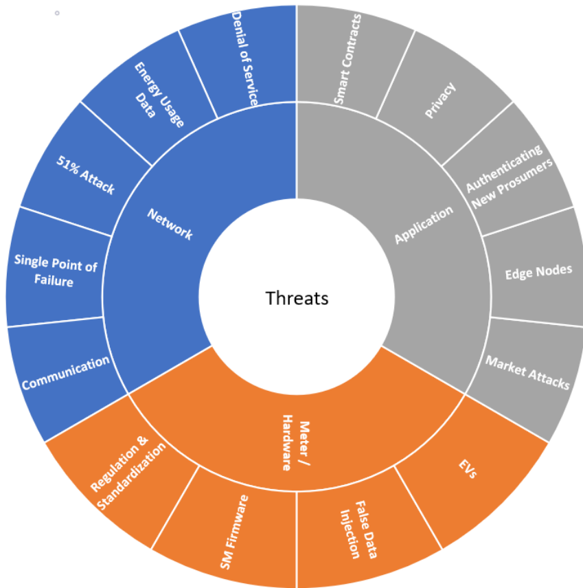
Figure 3.1: Simple taxonomy of the threats discovered. There are three overarching categories; the application layer, the network layer, and the hardware layer (including the smart meter itself). Each threat is relevant to at least one of these categories.
