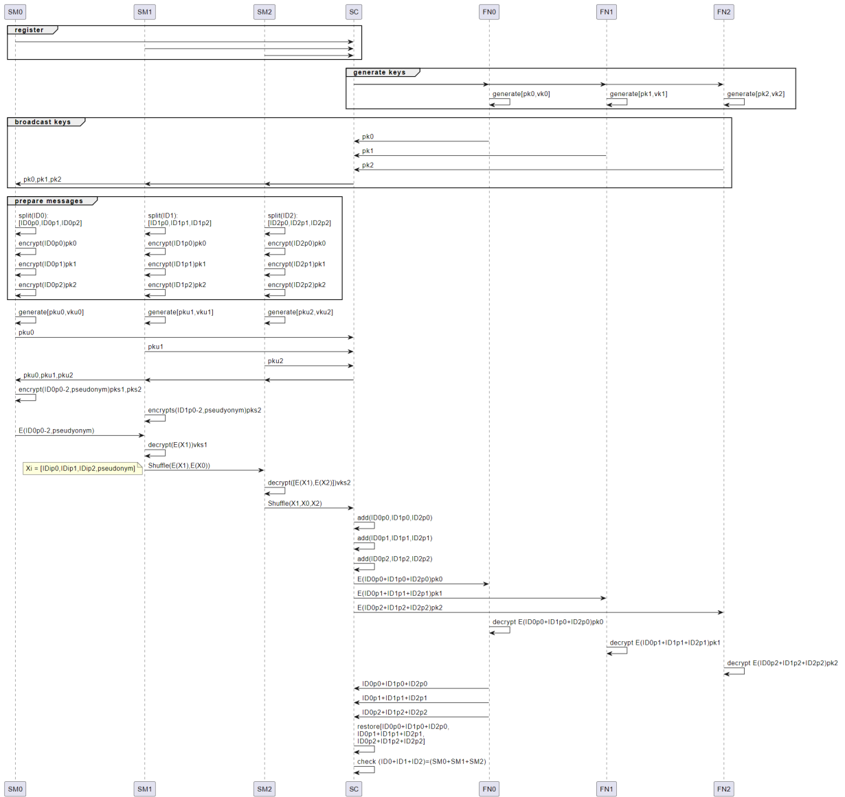
Figure 5.3: Full sequence diagram of the registration phase, operating on a batch of 3 users and 3 fog nodes.
