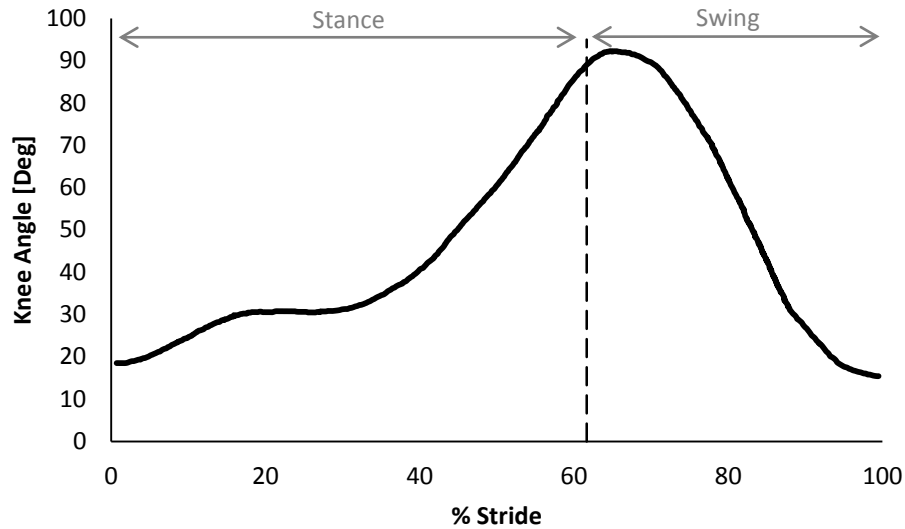
Figure 2.11: Knee joint angle for able-bodied stair descent for a typical step incline. Knee joint flexion is positive (reproduced from [17]).
