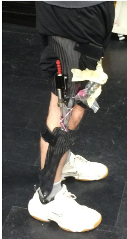
Figure 5.1: Participant wearing the carbon-fibre KAFO with the Ottawalk-Variable Speed orthotic joint on the lateral side and electronics taped to the front.
