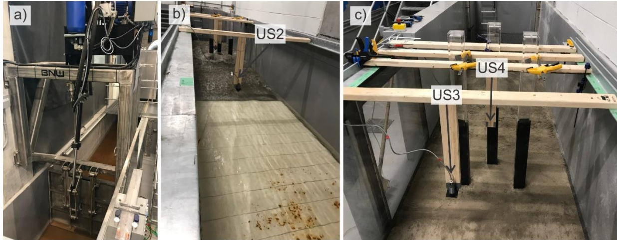
Figure 6.2: Pictures of experiment installation: a) swing gate system; b) false floor installation; c) measurement equipment and column support system
