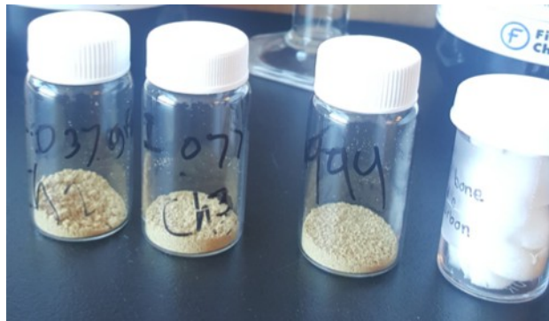
Figure 7 Photograph of examples of freeze-dried collagen extracted from chicken bones. Collagen extracted by NaOH or HCl method is white, whereas that extracted by KOH method is yellow.
