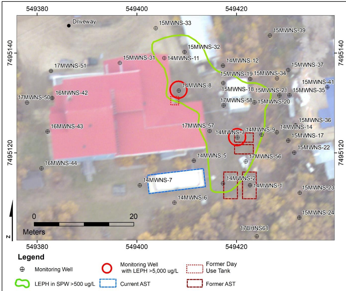
Figure 2.7 Interpreted extent of LEPH contaminants in supra-permafrost water at Old Crow Health Centre, Yukon based on Yukon Government contaminated site regulations (Air Photo from Yukon Government 2014, NAD83 UTM 7N)
