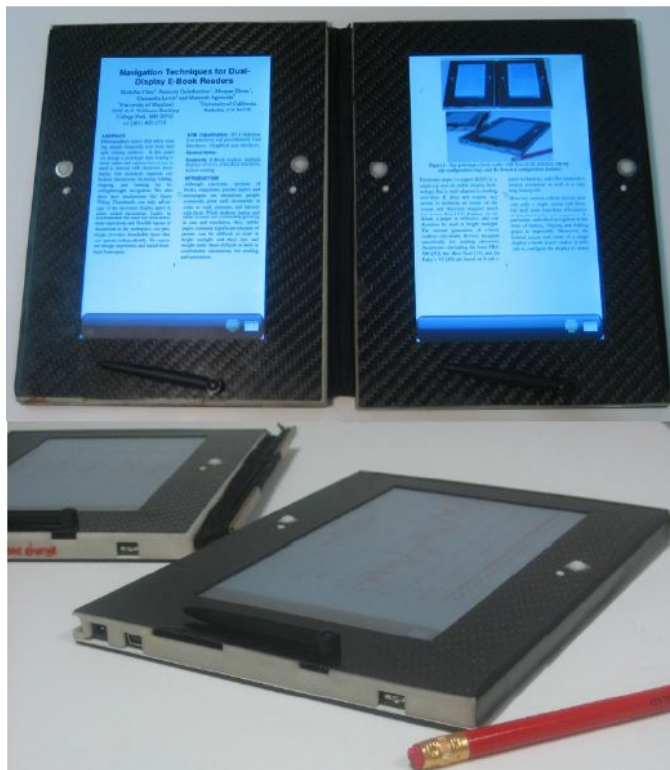
Figure 2.12: Prototype e-book reader with faces in the attached, side-by-side configuration (top), and the detached configuration (bottom). [15]
